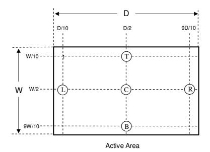
Luminance contrast is measured at the center point of the LCD panel "C" along with the normal of the display with the same distance described in Note 7. The display is then rotated around the vertical axis by changing its azimuthal axis to  $+30^{\circ}$ ; and this gives:
