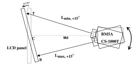
The LCD panel is then rotated to another azimuthal angle to -15°; and  $L_{min, -15^{\circ}}$  and  $L_{max, -15^{\circ}}$  are obtained by using the same procedure.
