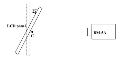
The LCD panel is then rotated to azimuthal angle to -30°; and  $L_{0 \text{ G} \text{ L}., -30^{\circ}}$  and  $L_{63 \text{ G} \text{ L}., -30^{\circ}}$  are obtained by using the same procedure. The Luminance Contrast is calculated:
