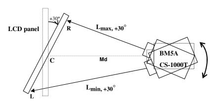
The LCD panel is then rotated to another azimuthal angle to -30°; and  $L_{min, -30}^{\circ}$  and  $L_{max, -30}^{\circ}$  are obtained by using the same procedure.
