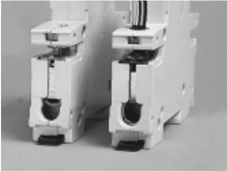
Dual function terminals provided in open position for connection to busbars. Pressing on screw head opens box terminal for cable insertion. Only the lower terminal is dual function.
