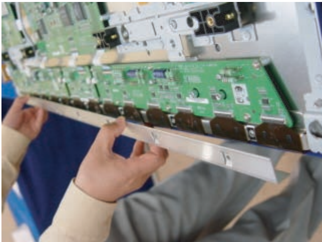
Figure 4-9 Photo 1 - Heatsink removal
