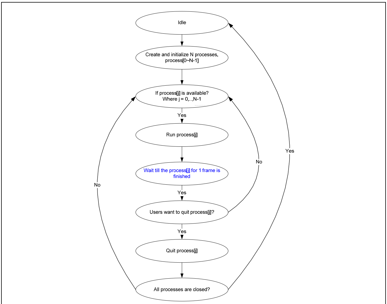
Figure 21-5. Codec firmware state diagram
