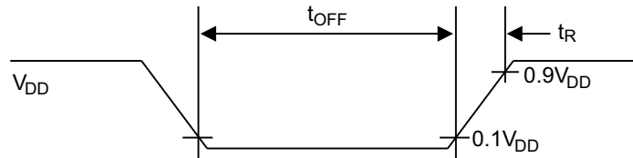
Figure 125. Low Voltage Reset Timing
