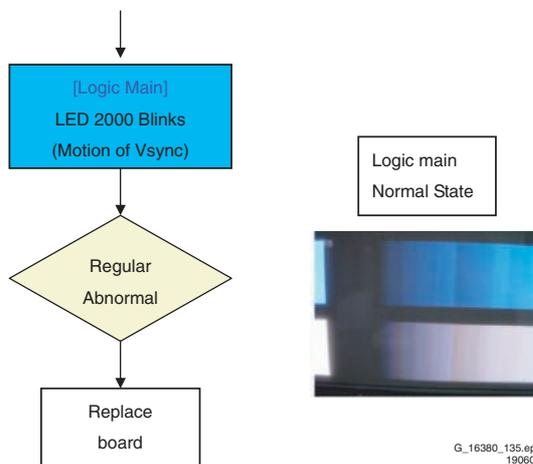
Figure 5-36 Fault symptom: "Abnormal Display" 42" SD v5 2/2
