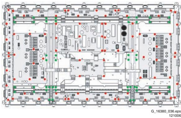
Figure 1-8 Location of mounting screws (63" HD v4)
