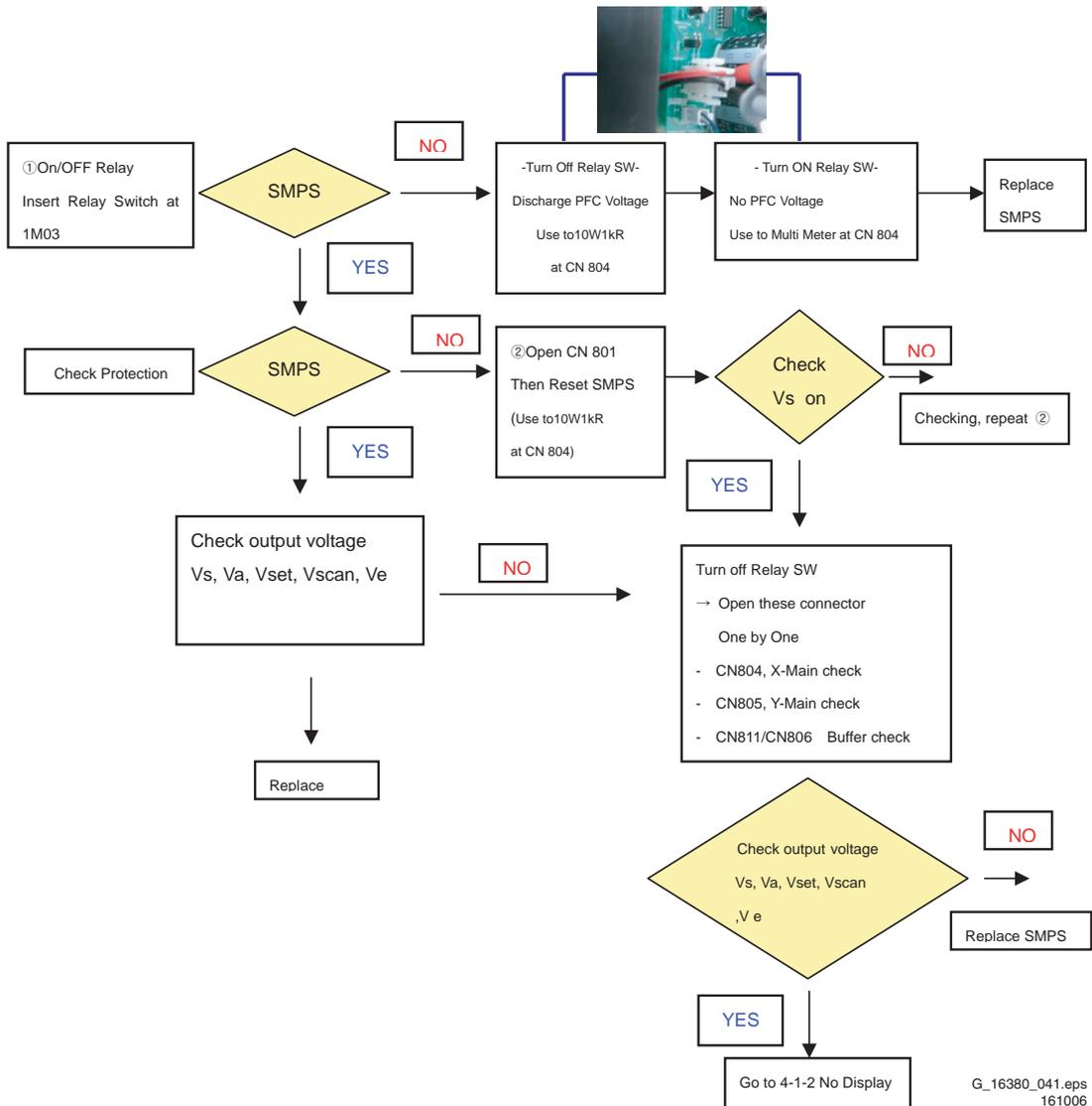
Figure 5-12 Power Supply Check for 63'' HD v4 models 2/2
