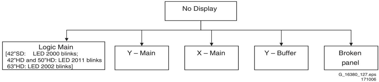
Figure 5-13 Fault symptom: "No Display", general guide line
