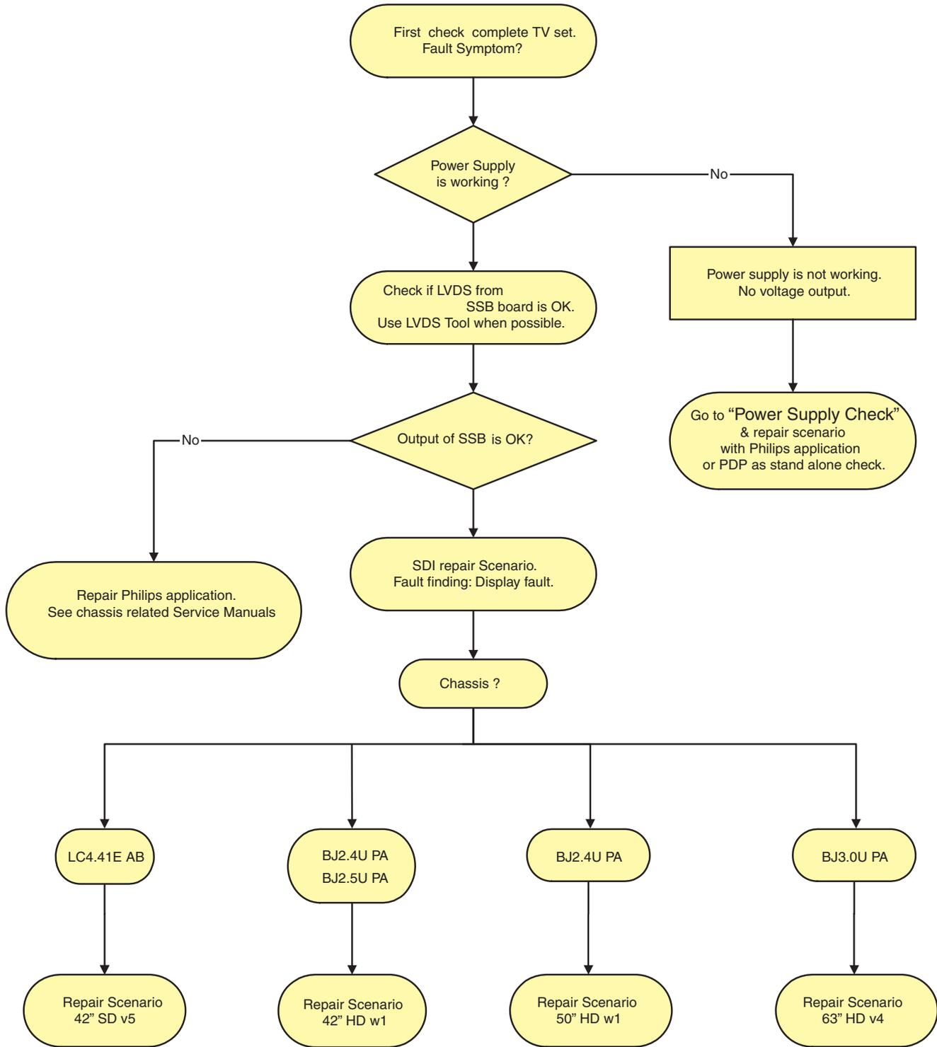
Figure 5-2 Which repair scenario?
