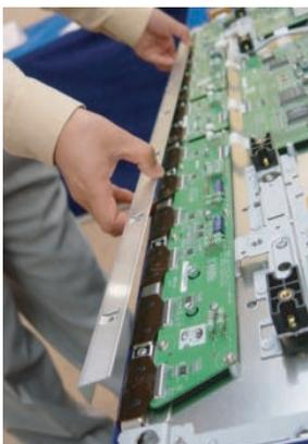
Figure 4-17 Photo 3 - Heat sink removal
