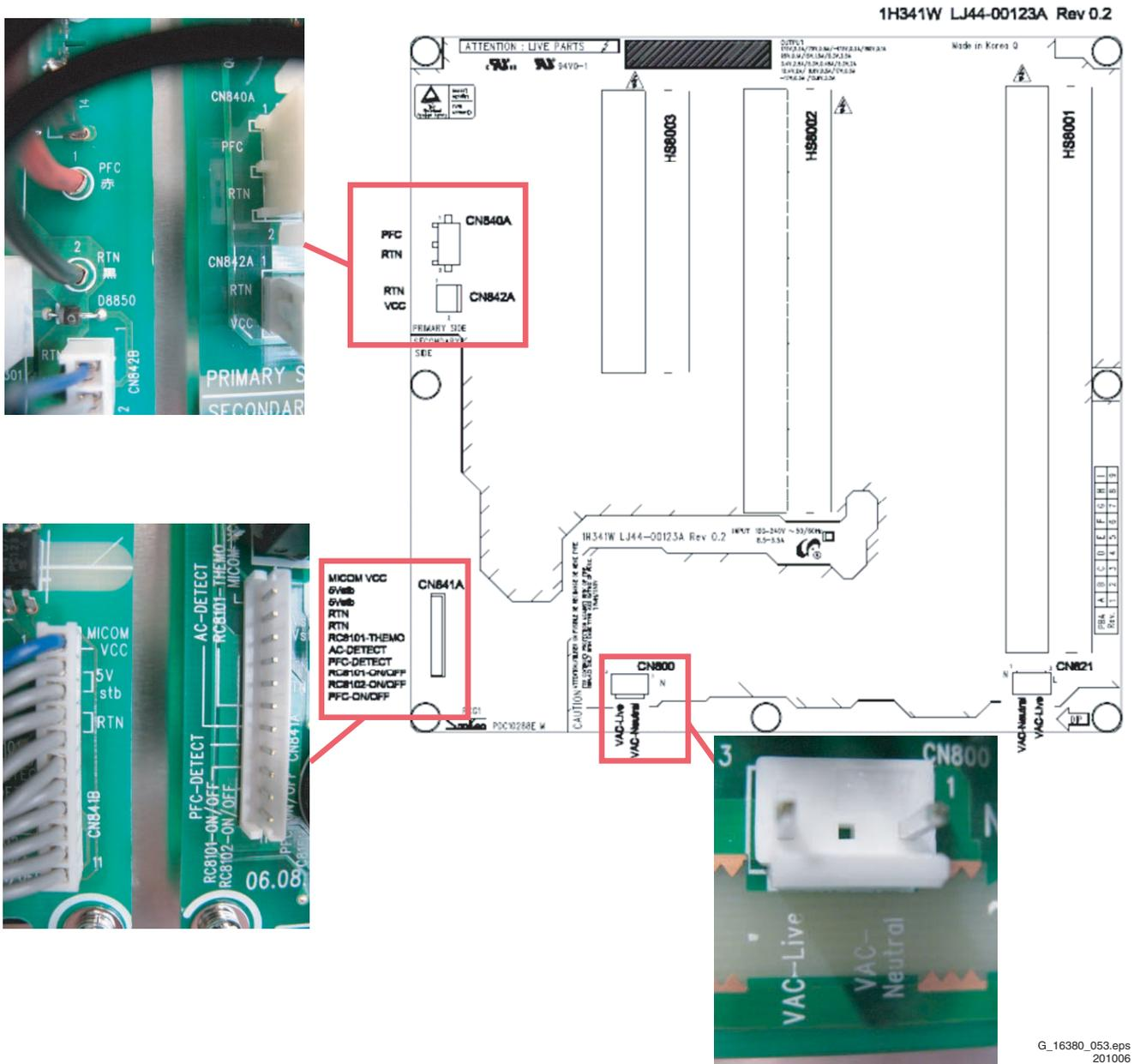
Figure 6-7 PSU layout (63" HD v4, Main PSU)
