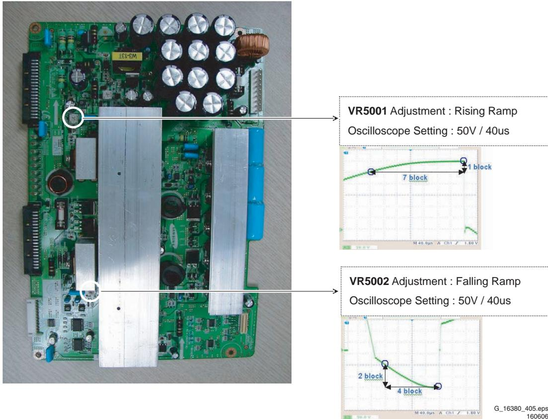
Figure 8-18 Adjusting procedure - 42" HD w1
