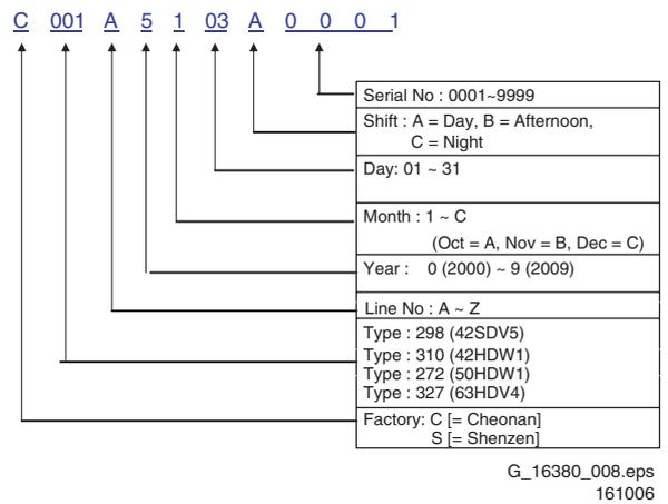
Figure 1-10 Explanation of the serial number
