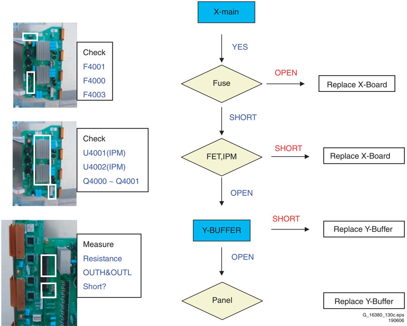
Figure 5-25 Fault symptom: “No Display”, 50” HD w1 4/6
