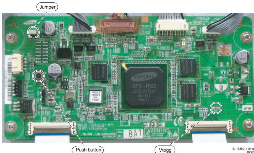
Figure 8-19 Logic PWB - 42" HD w1
