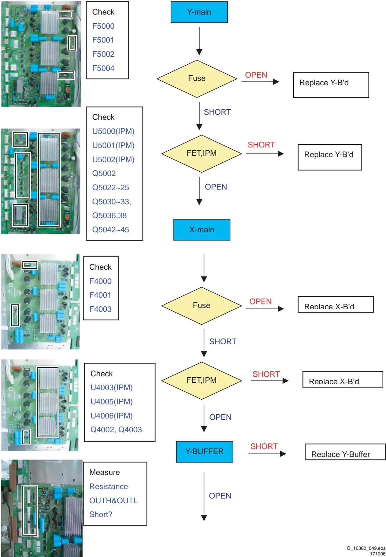
Figure 5-41 Fault symptom: "Abnormal Display" 63" HD v4 1/2
