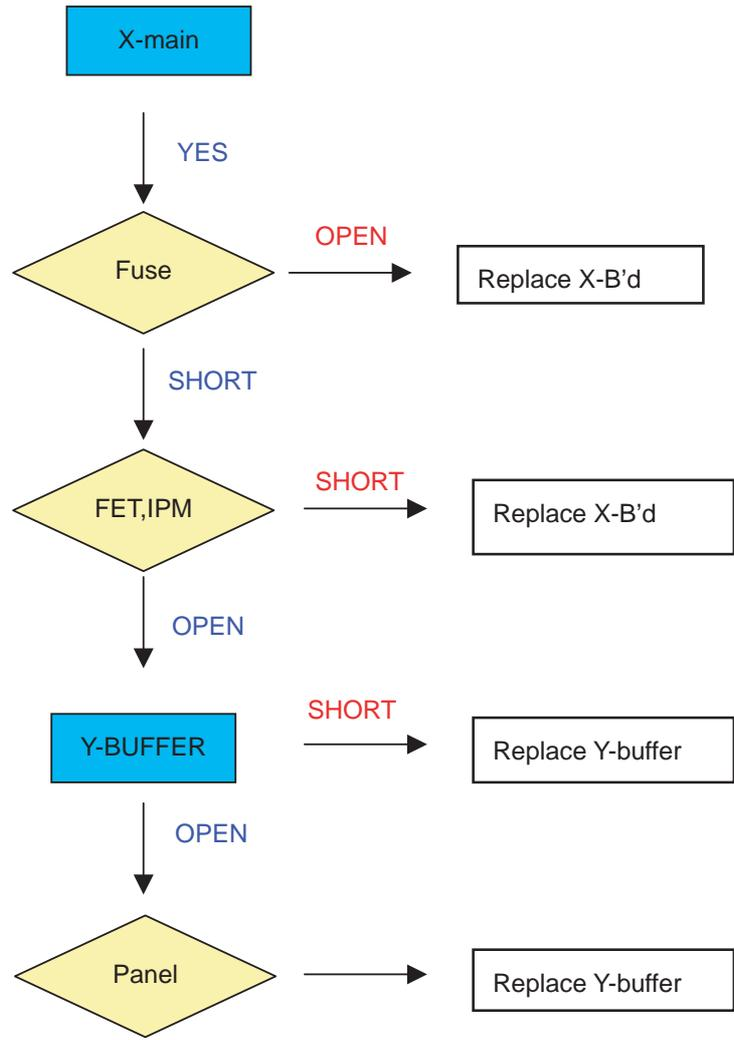
Figure 5-31 Fault symptom: "No Display", 63" HD v4 4/6
