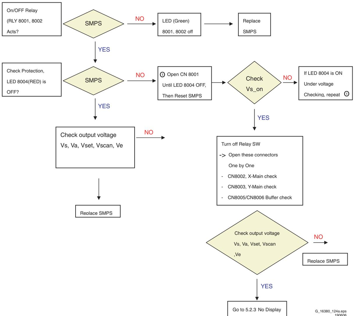
Figure 5-8 Power Supply Check for 42'' HD w1 models 2/2
