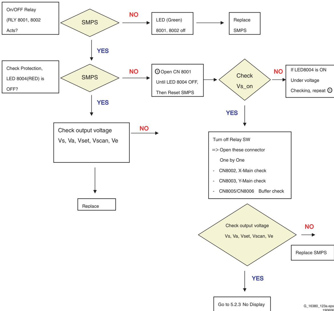
Figure 5-6 Power Supply Check for 42'' SD v5 models 2/2
