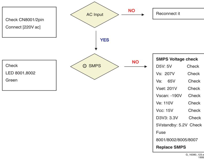
Figure 5-5 Power Supply Check for 42'' SD v5 models 1/2
