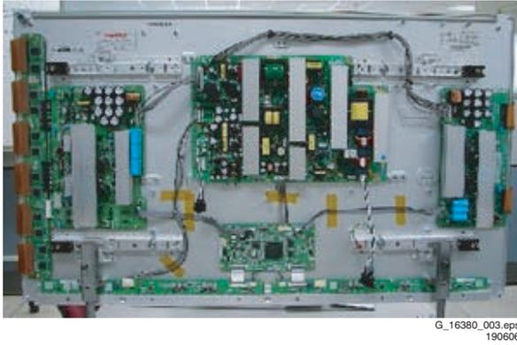
Figure 1-3 Rear view of plasma panel (42" HD w1)
