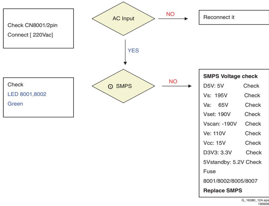
Figure 5-7 Power Supply Check for 42'' HD w1 models 1/2
