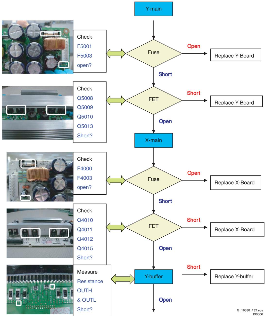
Figure 5-35 Fault symptom: "Abnormal Display" 42" SD v5 1/2
