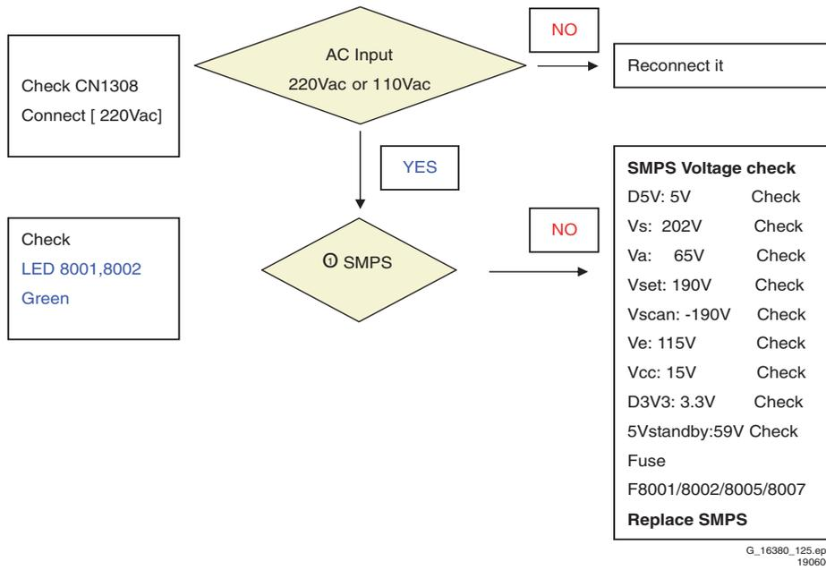
Figure 5-9 Power Supply Check for 50" HD w1 models 1/2
