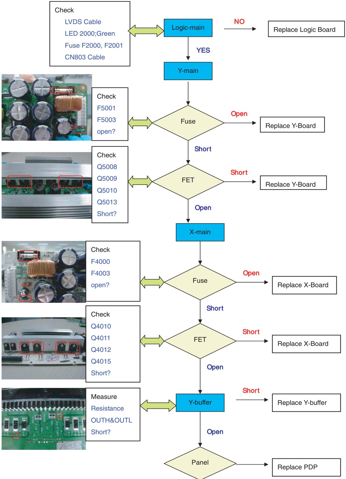
Figure 5-14 Fault symptom: "No Display", 42" SD v5
