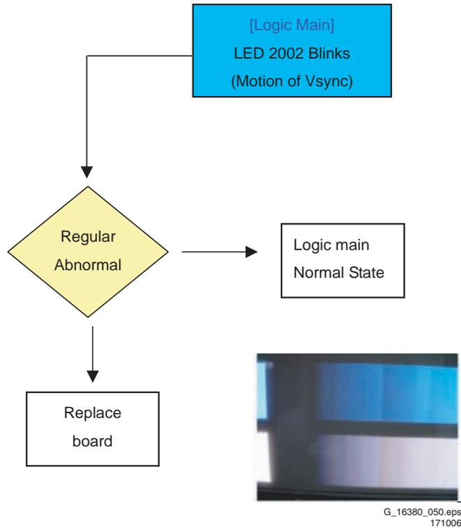
Figure 5-42 Fault symptom: "Abnormal Display" 63" HD v4 2/2
