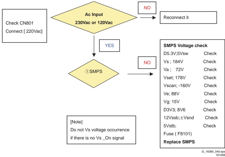
Figure 5-11 Power Supply Check for 63'' HD v4 models 1/2
