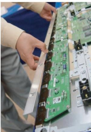
Figure 4-14 Photo 3 - Heat sink removal
