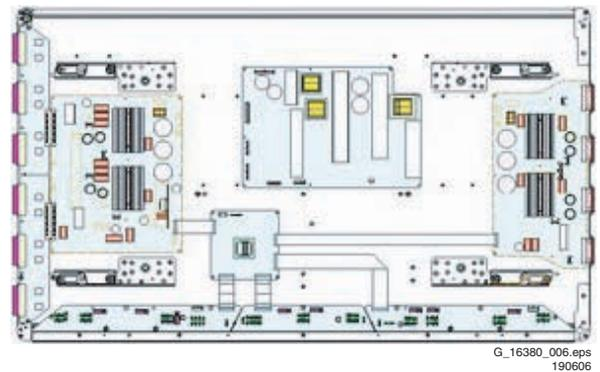
Figure 1-6 Location of mounting screws (50" HD w1)
