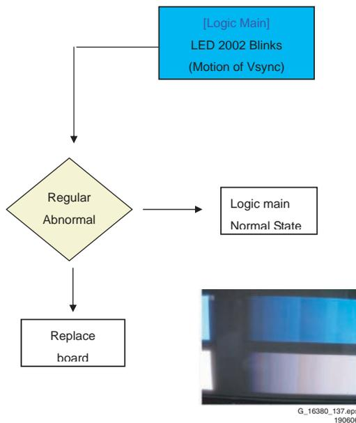
Figure 5-40 Fault symptom: "Abnormal Display" 50" HD w1 2/2
