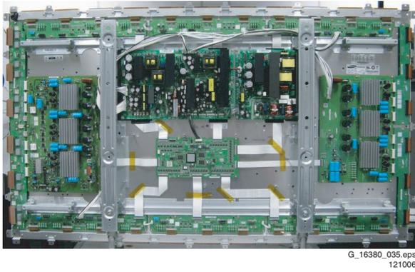
Figure 1-7 Rear view of plasma panel (63" HD v4)
