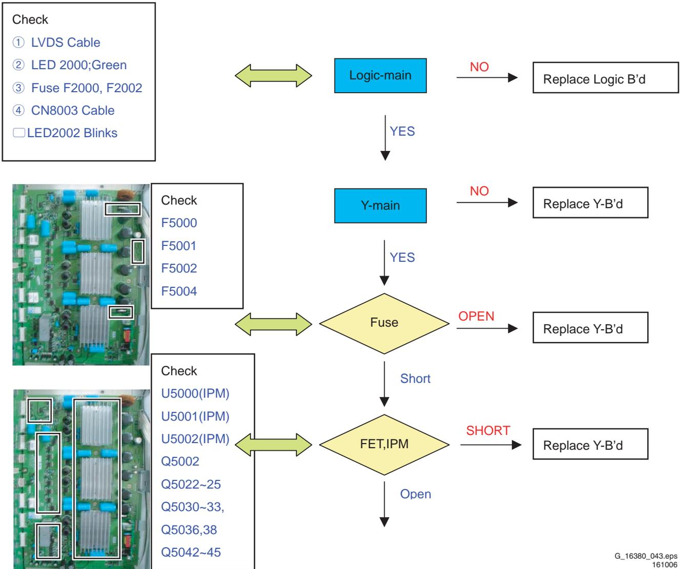
Figure 5-28 Fault symptom: "No Display", 63" HD v4 1/6
