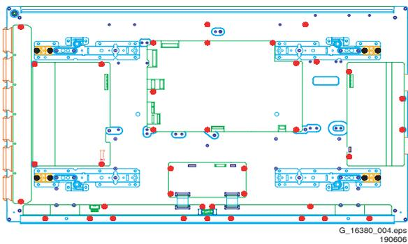
Figure 1-4 Location of mounting screws (42" HD w1)
