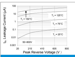
Fig.3 Typical Reverse Characteristics
