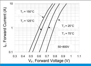
**Fig.5 Typical Forward Characteristics**
