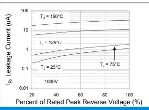
Fig.4 Typical Reverse Characteristics
