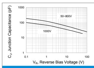
Fig.2 Typical Junction Capacitance
