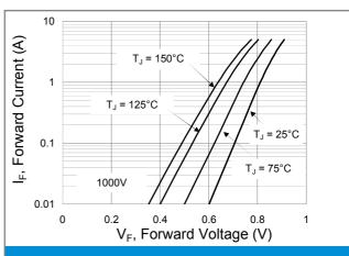
**Fig.6 Typical Forward Characteristics**
