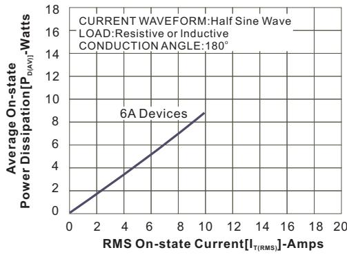
Figure E6.11 Power Dissipation (Typical) versus RMS On-state Current (6A)
