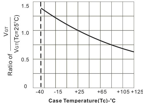
Figure E6.8 Normalized dc Gate-trigger Voltage versus Case Temperature
