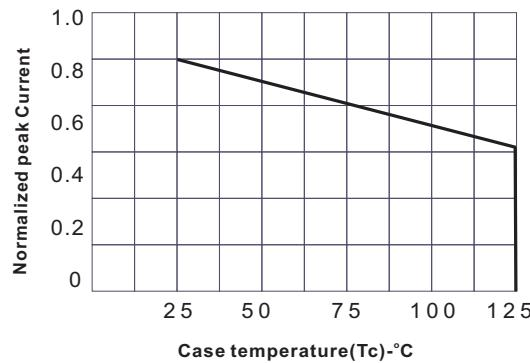
Figure E6.4 peak capacitor discharge current derating(6A)
