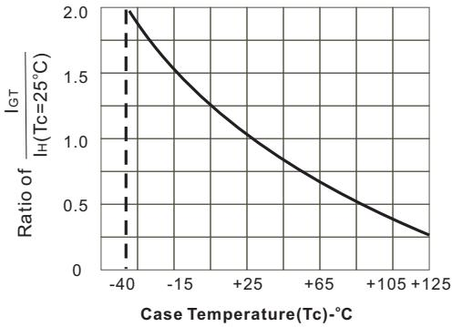
Figure E6.7 Normalized dc Gate-Trigger Current versus Case Temperature
