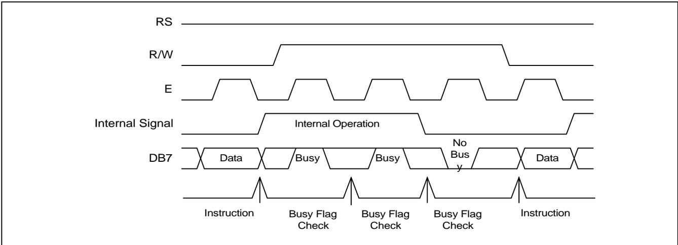
**Figure 11. Example of 8-bit Bus Mode Timing Sequence**
