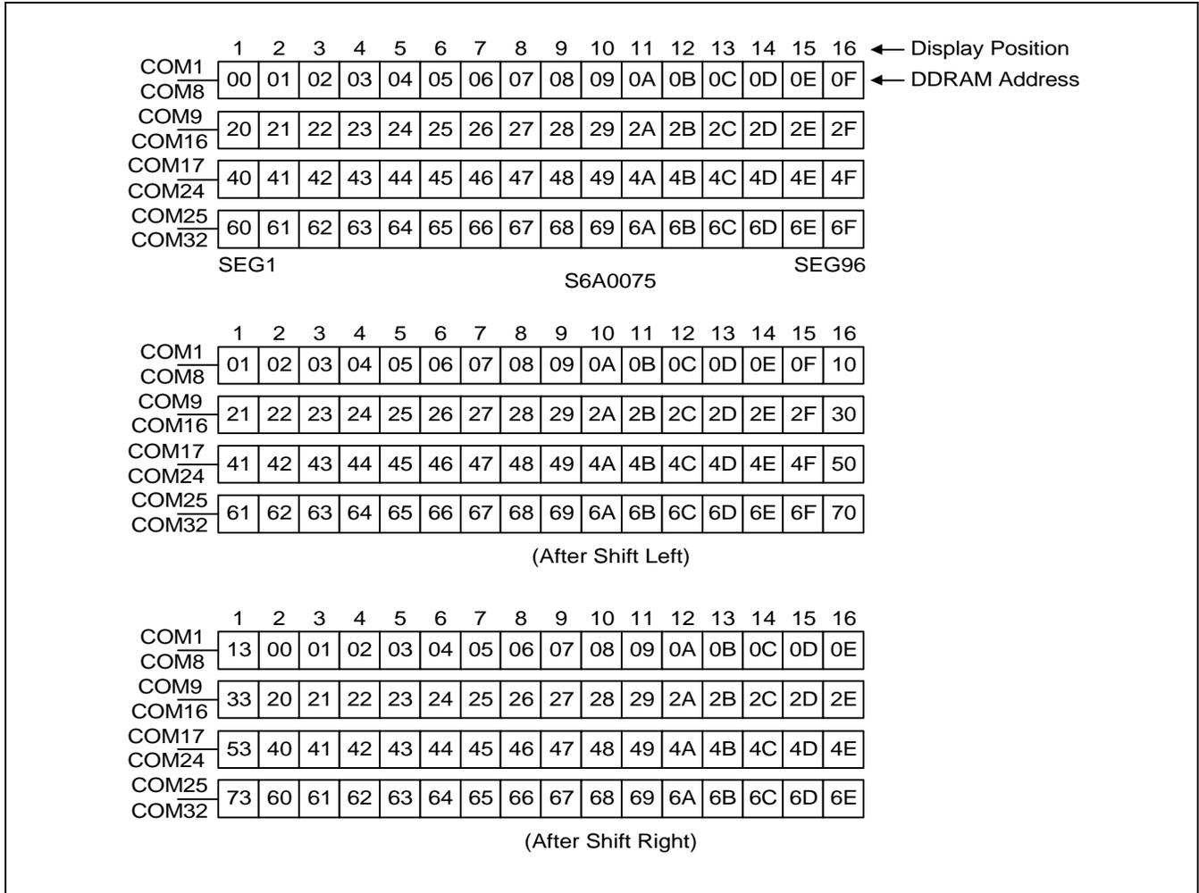
**Figure 7. 4-line × 16ch. Display (6-dot Font Width)**
