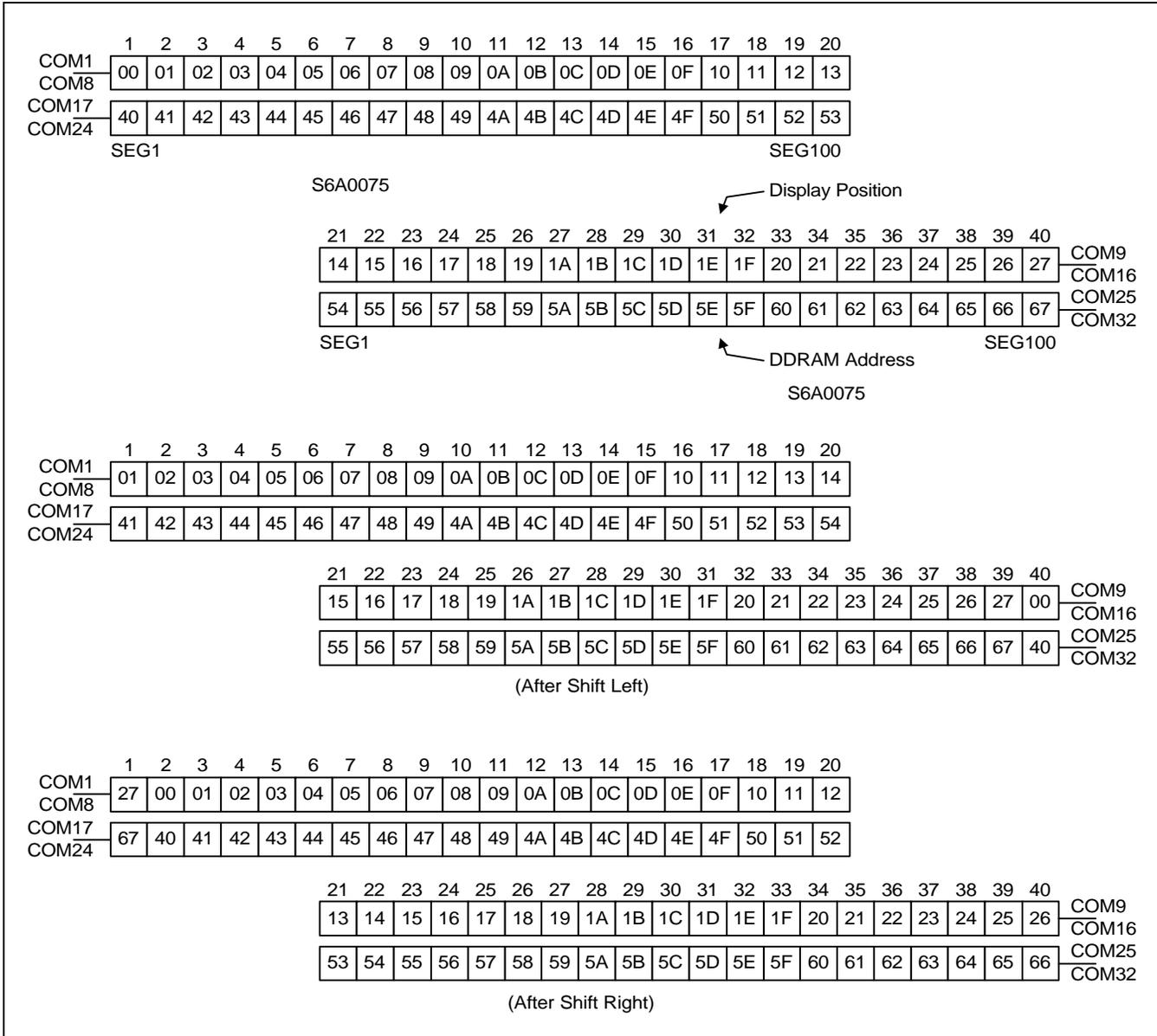
**Figure 3. 2-line x 40ch. Display (5-dot Font Width)**
