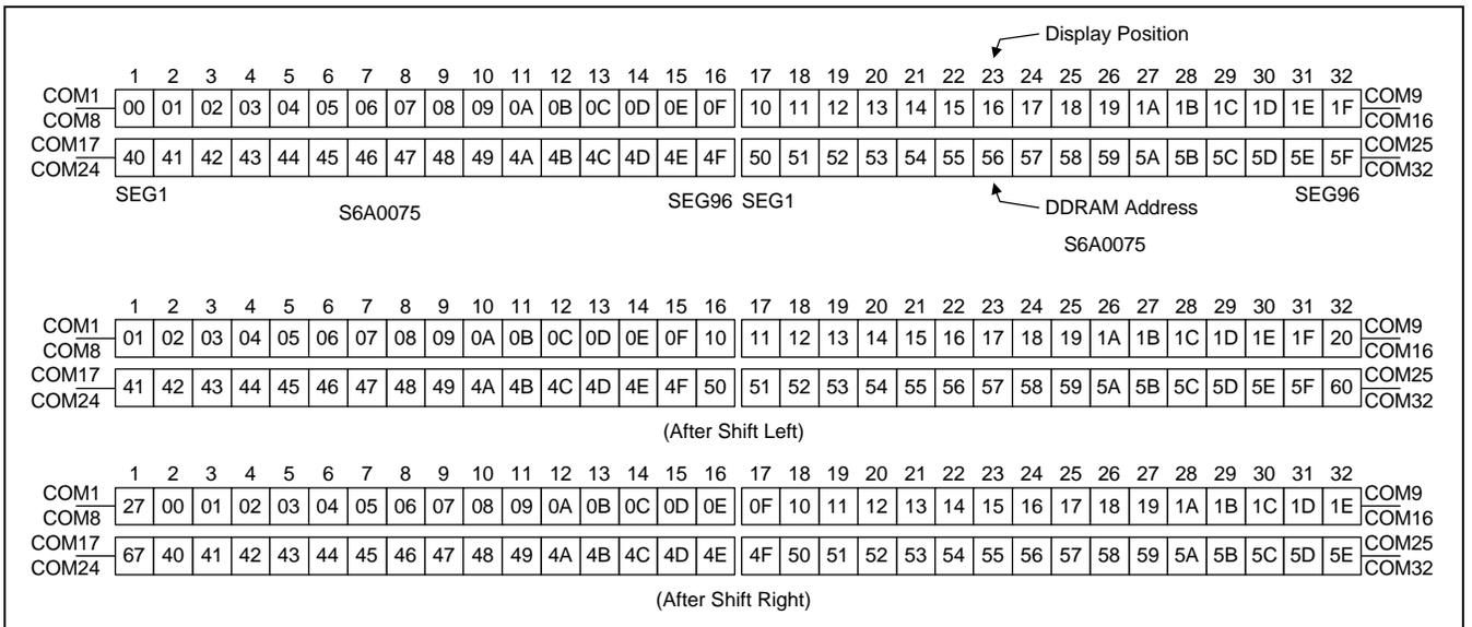
**Figure 6. 2-line x 32ch. Display (6-dot font width)**
