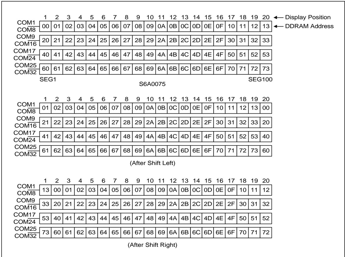
**Figure 4. 4-line x 20ch. Display (5-dot Font Width)**
