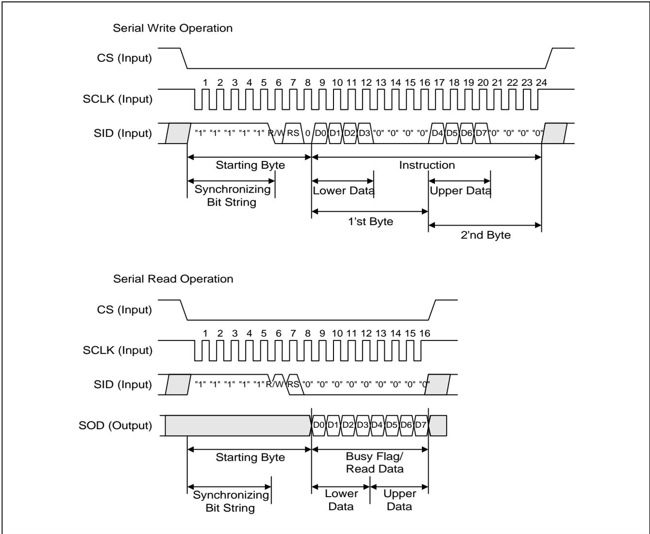
Figure 13. Timing Diagram of Serial Data Transfer
