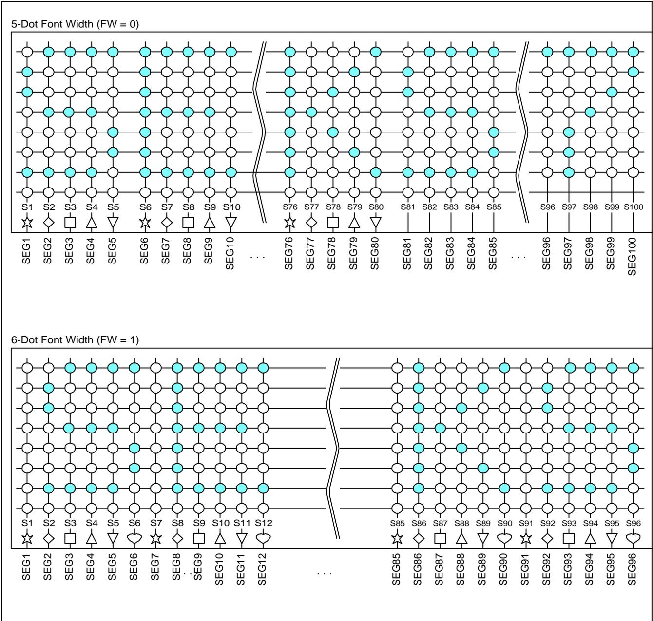
Figure 8. Relationship between SEGRAM and Segment Display
