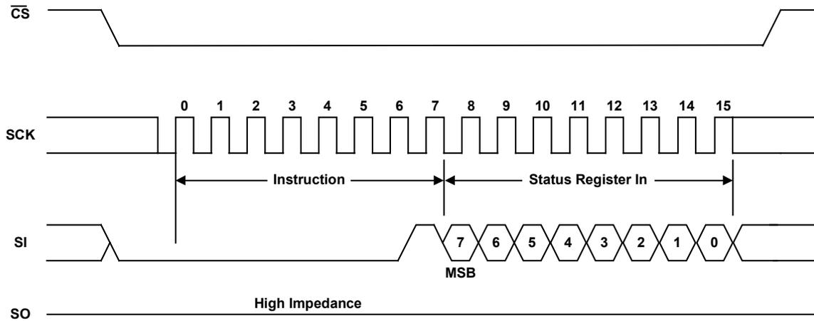
Figure 13. Write Status Register (WRSR) Instruction Sequence
