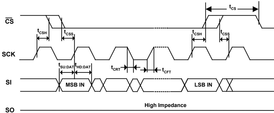
Figure 4. SPI Mode 0 (0,0) Input Timing
