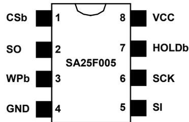
Figure 2. SOIC 8 (150 mil)/PDIP/MLF Package (Top View)
