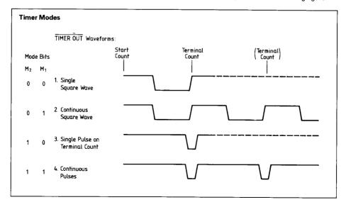
Bits 6–7 (TM2 and TM1) of command register contents are used to start and stop the counter. There are four commands to choose from:
