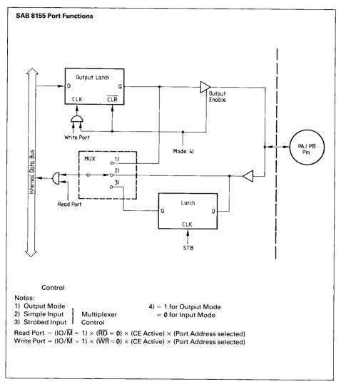
Note in the diagram that when the I/O ports are programmed to be output ports, the contents of the output ports can still be read by a READ operation when appropriately addressed.
