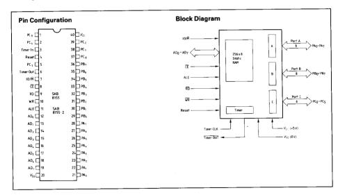
The SAB 8155 is a RAM and I/O chip to be used in the SAB 8085A and SAB 8088 microprocessor systems. The RAM portion is designed with 2048 static cells organized as 256×8. They have a maximum access time of 400ns to permit use with no wait states in SAB 8085A CPU. The SAB 8155-2 has a maximum access time of 330ns for use with the SAB 8085A-2 and the full speed 5MHz SAB 8088 CPU.
