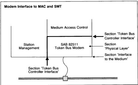
The interface (see figure above) provides the means for transferring information between the modem and the medium access control (MAC) and between the modem and the station management. In the interest of minimizing the number of signal lines, the station management uses the same lines as the MAC to access the modem. The interface supports three primary functions as described below:
