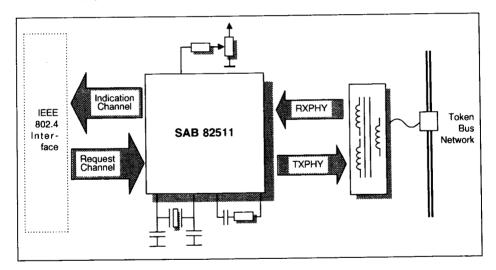
The token bus modem is designed to work directly with a token bus controller in IEEE 802.4 token bus applications. It uses phase-coherent frequency shift keying modulation at a data rate of 5 Mbit/s and 10 Mbit/s.
