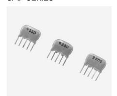
This series of SAW filters is designed for TV/VCR applications. These filters are capable of passing SIF, PIF, SIF or PIF. SAW filters are made up of zinc oxide on a glass substrate. Murata provides SAW filters for a variety of television standards world wide.
