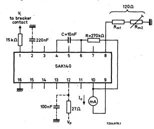
Temperature coefficient of  $\rm I_{\rm O}$  is 800 ppm/°C determined by an internal diode between pins 7 and 8.  $^{\rm I})$
