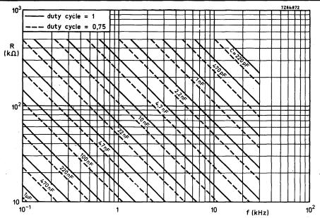
For other duty cycles at f. s.d. than  $\theta$ , 75, the value of R or C derived from the graph at a duty cycle of 1 must be multiplied by the duty cycle required.
