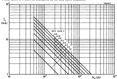
If a diode is connected in series with  $\mathbf{R}_m$  , the value of  $\mathbf{R}_m$  derived from the graph must be lowered with 25 %.
