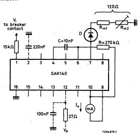
Temperature coefficient of I<sub>o</sub> is 800 ppm/°C determined by diode D. <sup>1</sup>)
