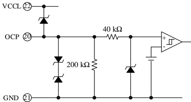
Figure 8-4. Internal Circuit Diagram of OCP Pin
