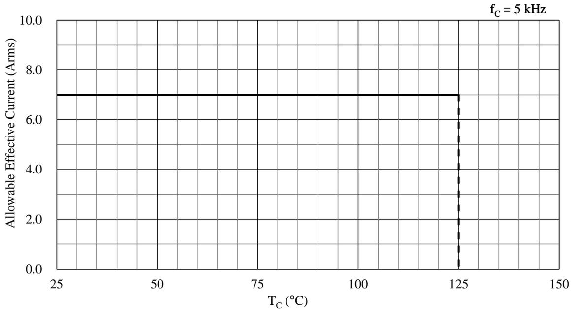
Figure 16-6. Allowable Effective Current ( $f_C = 5$  kHz)
