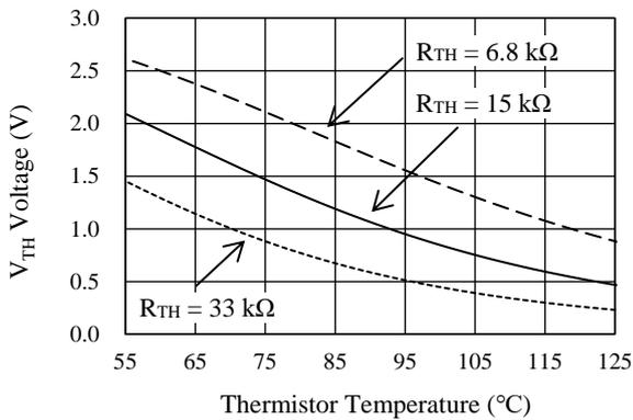
Figure 13-10. V<sub>TH</sub> Voltage vs. Thermistor Temperature (V<sub>TH\_PU</sub> = 3.3 V)
