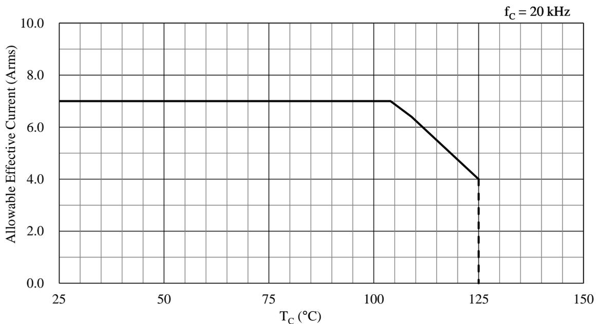
Figure 16-7. Allowable Effective Current ( $f_C = 20$  kHz)
