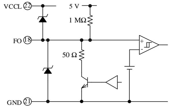
Figure 8-3. Internal Circuit Diagram of FO Pin
