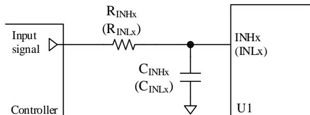
Figure 13-6. Filter Circuit for INHx or INLx Pin
