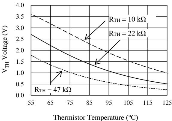
Figure 13-11. V<sub>TH</sub> Voltage vs. Thermistor Temperature (V<sub>TH\_PU</sub> = 5.0 V)
