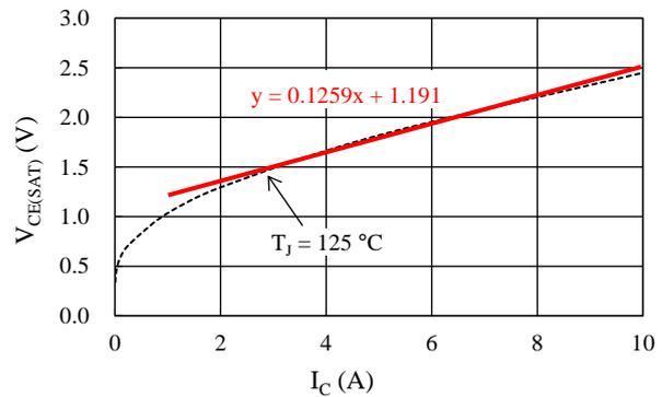
Figure 15-1. Linear Approximate Equation of  $V_{CE(SAT)}$  vs.  $I_C$
