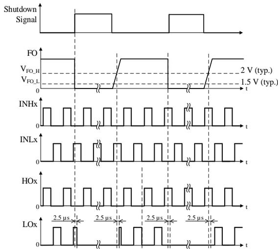
Figure 13-12. Operational Waveforms at Shutdown Signal Input
