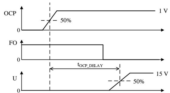
Figure 4-2. OCP Pin Detection Delay Time Definition
