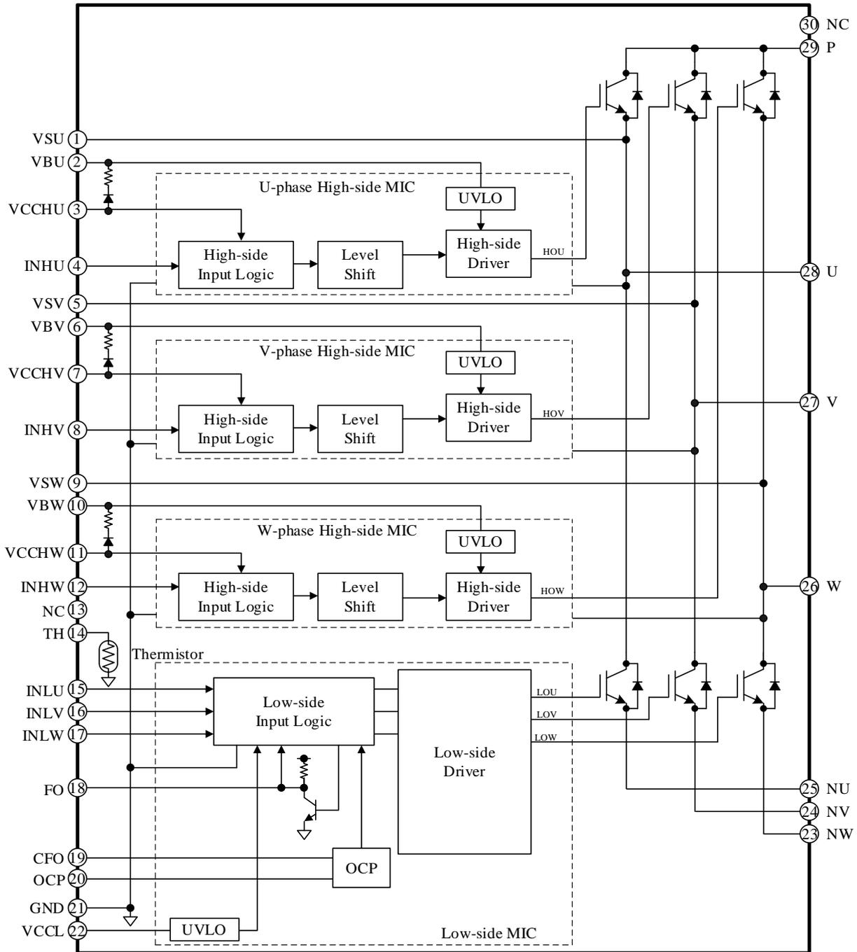
Figure 8-1. Block Diagram
