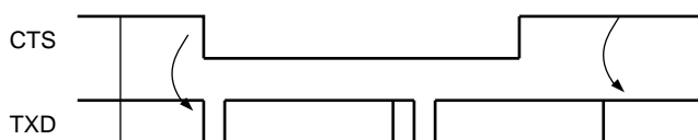
Figure 34-29. Transmitter Behavior when Operating with Hardware Handshaking
