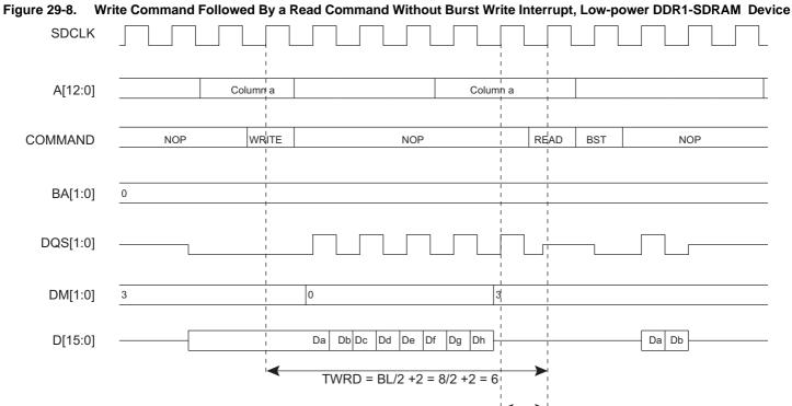
In the case of a single write access, write operation should be interrupted by a read access but DM must be input 1 cycle prior to the read command to avoid writing invalid data. (See Figure 29-9.)
