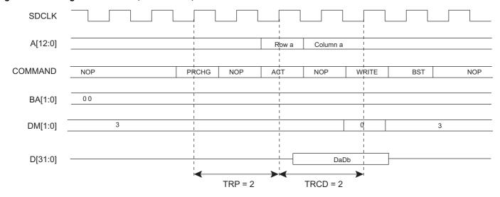
Figure 29-5. Burst Write Access, Row Closed, Low-power DDR1-SDRAM Device
