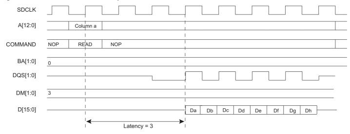
Figure 29-16. Burst Read Access, Latency = 2, SDR-SDRAM Devices
