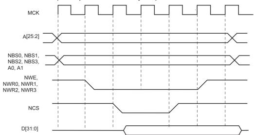
Figure 28-15. WRITE\_MODE = 0 (Write Operation Controlled by NCS)
