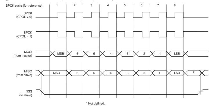
Figure 34-4. SPI Transfer Format (NCPHA = 0, 8 bits per transfer)
