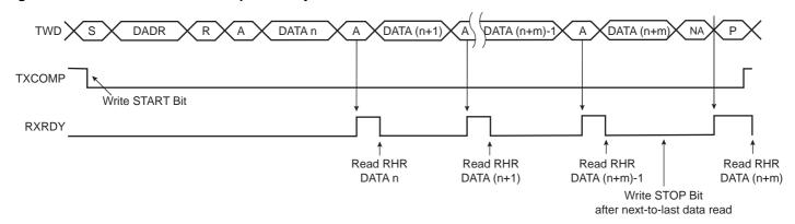
Figure 37-9. Master Read Wait State with Multiple Data Bytes
