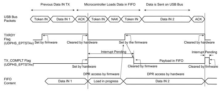
Figure 31-10. Data IN Transfer for Endpoint with Two Banks
