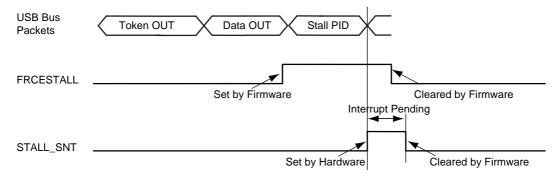
Figure 31-18. Stall Handshake Data IN Transfer
