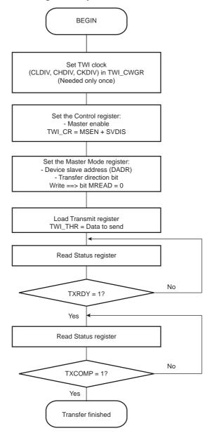
Figure 37-14. TWI Write Operation with Single Data Byte and Internal Address
