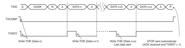
Figure 37-6. Master Write with One Byte Internal Address and Multiple Data Bytes
