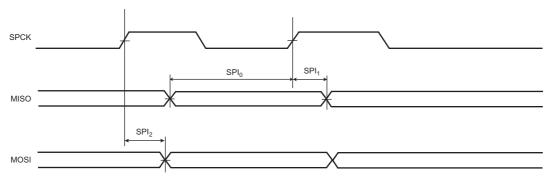
Figure 45-11. SPI Master mode 0 and 3
