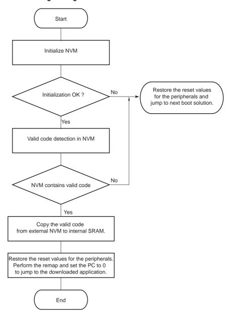
The NVM bootloader program first initializes the PIOs related to the NVM device. Then it configures the right peripheral depending on the NVM and tries to access this memory. If the initialization fails, it restores the reset values for the PIO and the peripheral and then tries the same operations on the next NVM of the sequence.
