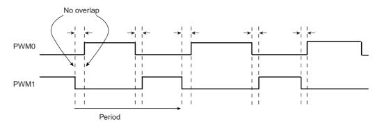
Note: See Figure 36-5 on page 752 for a detailed description of center aligned waveforms.
