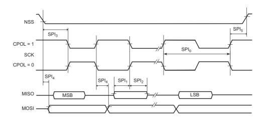
Figure 45-30. USART SPI Slave mode: (Mode 1 or 2)
