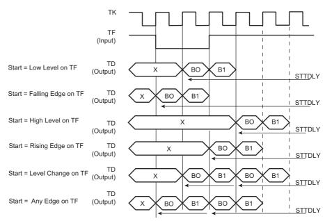
Figure 42-14. Receive Pulse/Edge Start Modes
