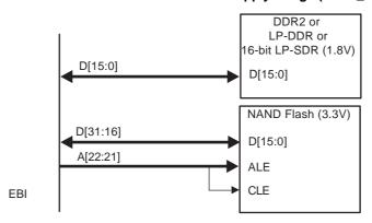
At reset NFD0\_ON\_D16 = 0 and the NAND Flash bus is connected to D0-D15.
