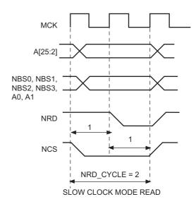
Table 28-6. Read and Write Timing Parameters in Slow Clock Mode
