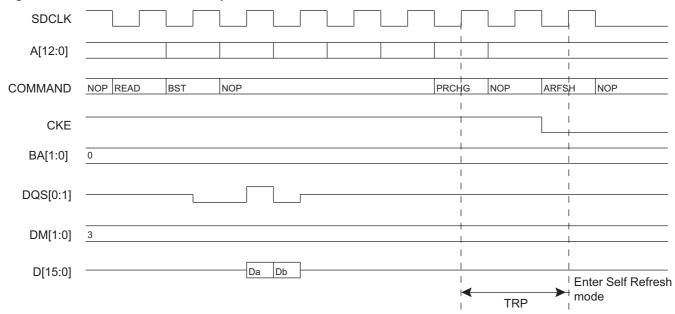
Figure 29-18. Self Refresh Mode Entry, DDRSDRC\_LPR.TIMEOUT = 1 or 2
