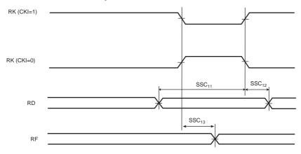
Figure 45-23. SSC Receiver, RK in ouput and RF in Input
