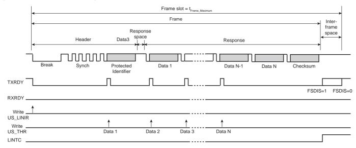
Figure 38-46. Master Node Configuration, NACT = SUBSCRIBE
