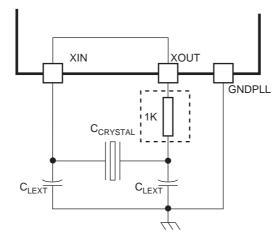
Note: A 1K resistor must be added on XOUT pin for crystals with frequencies lower than 8 MHz.
