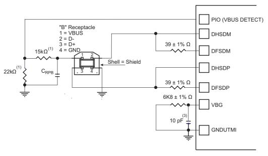
Notes: 1. The values shown on the 22 k $\Omega$  and 15 k $\Omega$  resistors are only valid with 3V3-supplied PIOs. Both 39  $\Omega$  resistors need to be placed as close to the device pins as possible.
