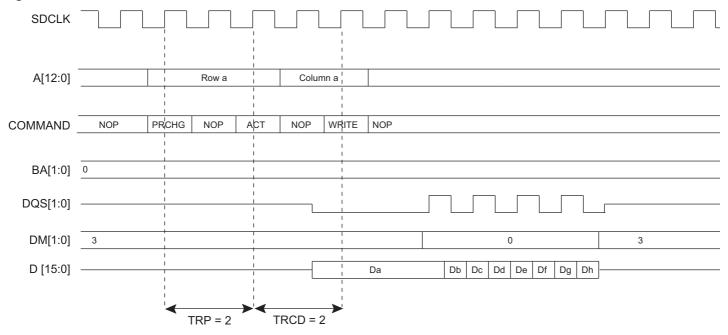
Figure 29-7. Burst Write Access, Row Closed, SDR-SDRAM Device
