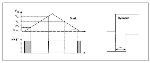
When a very slow (versus  $t_{RES}$ ) supply rising slope is applied on POR VDD pin, the reset time becomes negligible and the reset signal is released when  $V_{DD}$  rises higher than  $V_{th+}$ .
