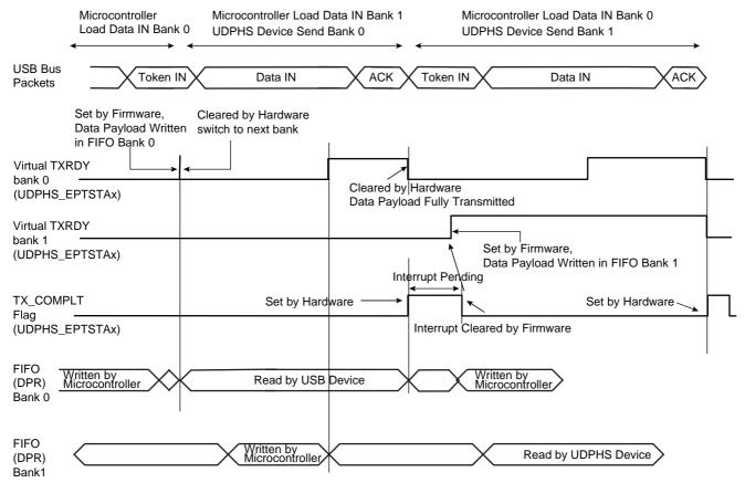
Figure 31-11. Data IN Followed By Status OUT Transfer at the End of a Control Transfer
