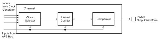
Each of the 4 channels is composed of three blocks:
