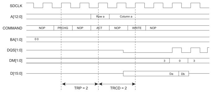
Figure 29-4. Single Write Access, Row Closed, SDR-SDRAM Device
