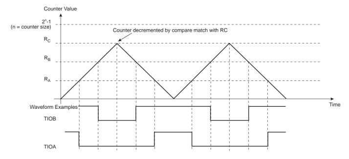
Figure 35-14. WAVSEL = 11 with Trigger
