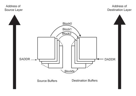
Figure 30-10. DMAC Transfer Flow for Source and Destination Address Auto-reloaded
