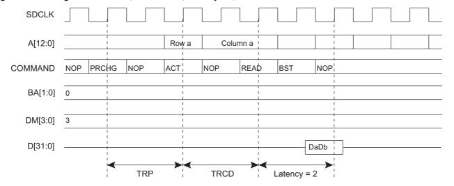
Figure 29-14. Burst Read Access, Latency = 2, Low-power DDR1-SDRAM Devices
