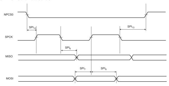
Figure 45-13. SPI Slave mode 1 and 2
