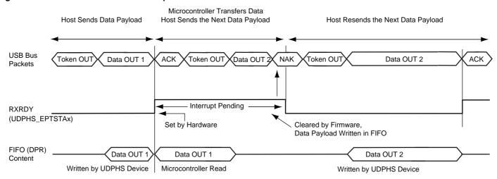
Figure 31-15. Data OUT Transfer for an Endpoint with Two Banks
