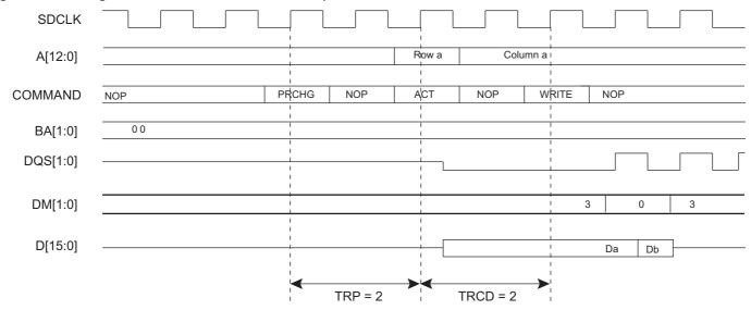
Figure 29-3. Single Write Access, Row Closed, DDR2-SDRAM Device
