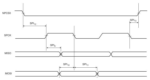
Figure 45-14. SPI Slave mode - NPCS timings
