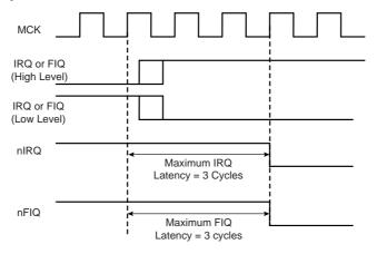
Figure 12-8. Internal Interrupt Edge Triggered Source
