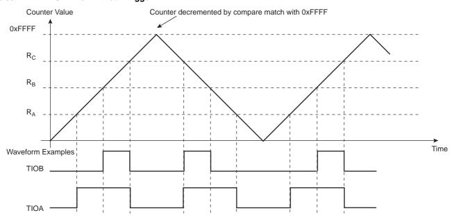
Figure 35-12. WAVSEL = 01 with Trigger
