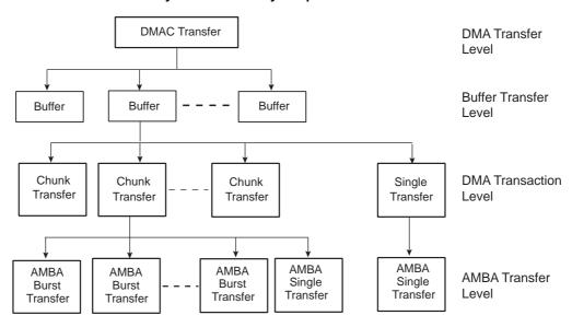
Figure 30-3. DMAC Transfer Hierarchy for Memory
