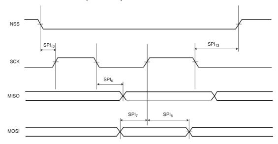
Figure 45-31. USART SPI Slave mode: (Mode 0 or 3)
