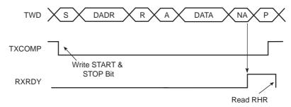
Figure 37-8. Master Read with Multiple Data Bytes
