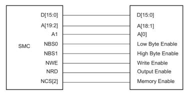
Figure 28-5. Memory Connection for a 32-bit Data Bus
