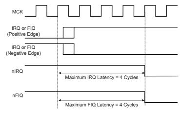
Figure 12-7. External Interrupt Level Sensitive Source
