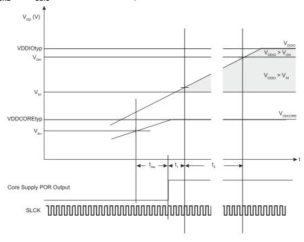
$V_{\text{DDCORE}}$  and  $V_{\text{DDBU}}$  are controlled by internal POR (Power-On-Reset) to guarantee that these power sources reach their target values prior to the release of POR.
