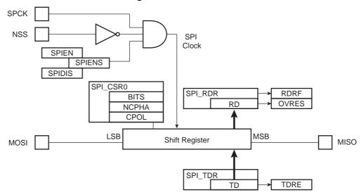
Figure 34-12. Slave Mode Functional Block Diagram
