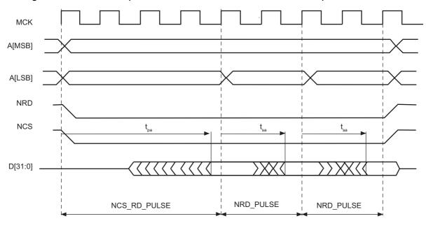
The NRD and NCS signals are held low during all read transfers, whatever the programmed values of the setup and hold timings in the User Interface may be. Moreover, the NRD and NCS timings are identical. The pulse length of the first access to the page is defined with the NCS\_RD\_PULSE field of the SMC\_PULSE register. The pulse length of subsequent accesses within the page are defined using the NRD\_PULSE parameter.
