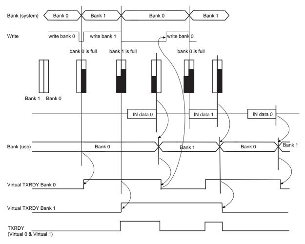
Note: In the illustration above Autovalid validates a bank as full, although this might not be the case, in order to continue processing data and to send to DMA.
