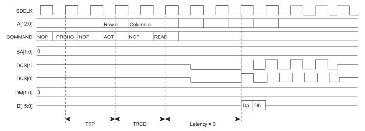
Figure 29-13. Single Read Access, Row Closed, Latency = 2, SDR-SDRAM Device
