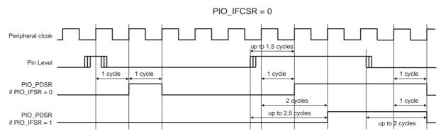
Figure 22-5. Input Debouncing Filter Timing
