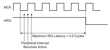
Figure 12-9. Internal Interrupt Level Sensitive Source
