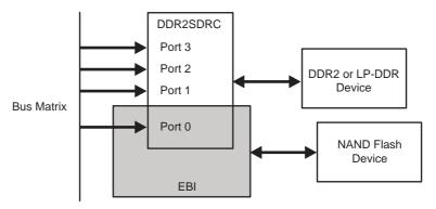
Figure 25-5. DDR2SDRC Multi-port Disabled (DDR\_MP\_EN = 0)
