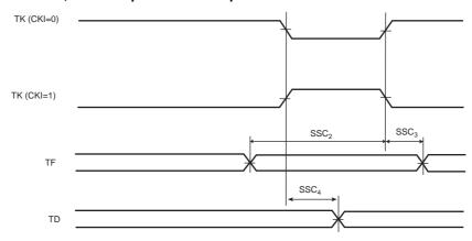
Figure 45-19. SSC Transmitter, TK and TF in Input
