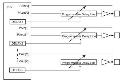
Figure 22-8. Programmable I/O Delays
