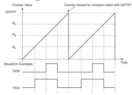
Figure 35-8. WAVSEL = 00 with Trigger
