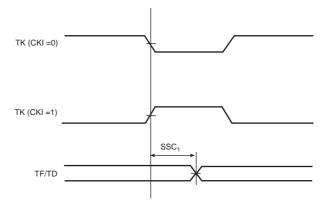
Figure 45-18. SSC Transmitter, TK in Output and TF in Input
