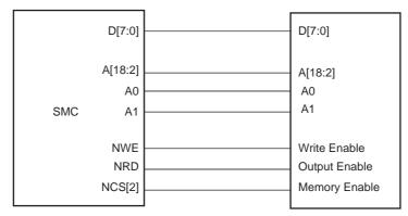
Figure 28-4. Memory Connection for a 16-bit Data Bus
