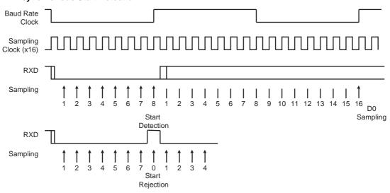
Figure 38-12. Asynchronous Character Reception
