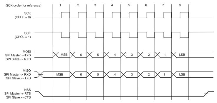
Figure 38-38. SPI Transfer Format (CPHA = 0, 8 bits per transfer)
