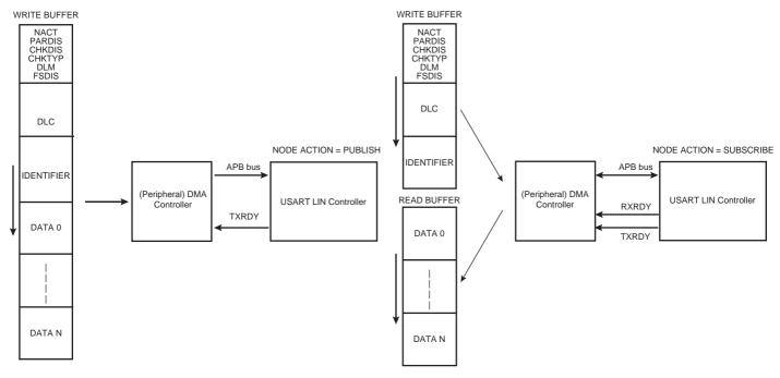
Figure 38-52. Master Node with DMAC (PDCM = 0)
