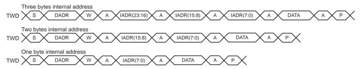
Figure 37-11. Master Read with One, Two or Three Bytes Internal Address and One Data Byte
