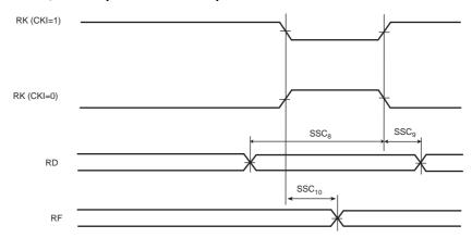
Figure 45-22. SSC Receiver, RK and RF in Output
