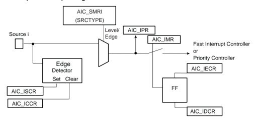
Figure 12-5. External Interrupt Source Input Stage
