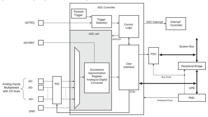
Note: DMA may be referred to as PDC (Peripheral DMA Controller).
