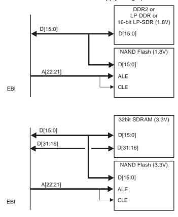
Figure 25-3 illustrates an example of the NAND Flash and the external RAM (DDR2 or LP-DDR or 16-bit LP-SDR) **not** in the same power supply range (NFD0\_ON\_D16 = 1).
