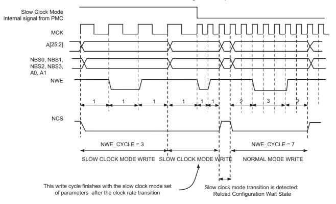
Figure 28-33. Recommended Procedure to Switch from Slow Clock Mode to Normal Mode or from Normal Mode to Slow Clock Mode
