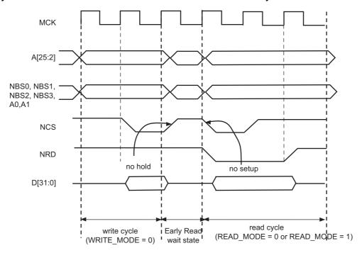
Figure 28-19. Early Read Wait State: NWE-controlled Write with No Hold Followed by a Read with one Set-up Cycle
