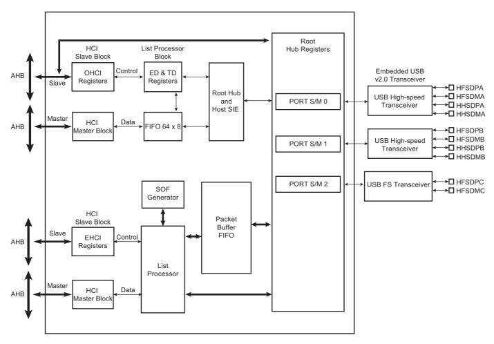
Access to the USB host operational registers is achieved through the AHB bus slave interface. The Open HCI host controller and Enhanced HCI host controller initialize master DMA transfers through the AHB bus master interface as follows:
