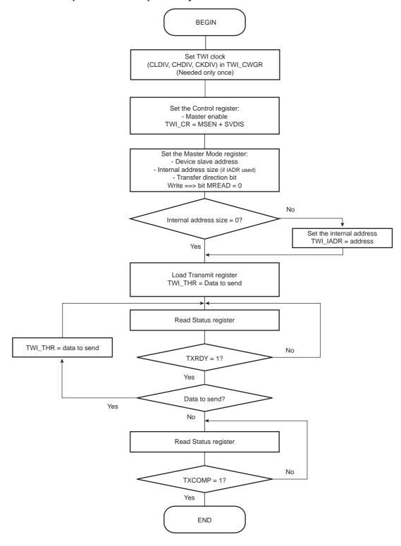
Figure 37-16. TWI Read Operation with Single Data Byte without Internal Address
