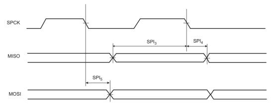
Figure 45-12. SPI Slave mode 0 and 3
