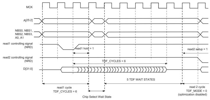
Figure 28-24. TDF Mode = 0: TDF wait states between a read and a write access on different chip selects
