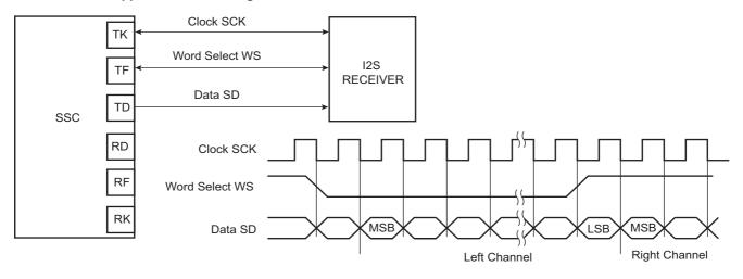
Figure 42-4. Codec Application Block Diagram
