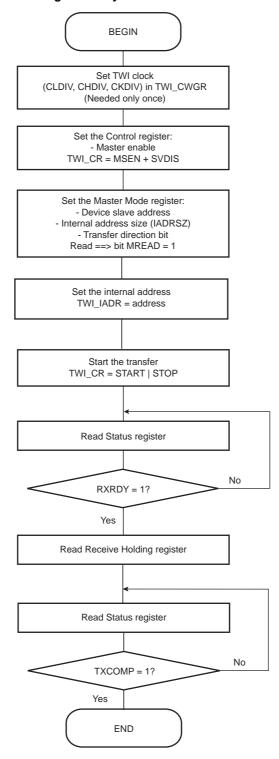
Figure 37-18. TWI Read Operation with Multiple Data Bytes with or without Internal Address
