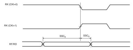
Figure 45-21. SSC Receiver, RK in Input and RF in Output
