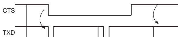
Figure 43-28. Transmitter Behavior when Operating with Hardware Handshaking
