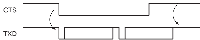
Figure 43-28. Transmitter Behavior when Operating with Hardware Handshaking
