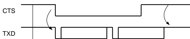
Figure 30-19. Transmitter Behavior when Operating with Hardware Handshaking
