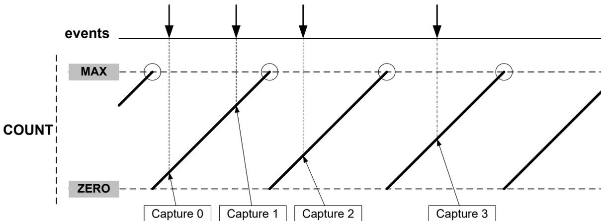
For input capture, the buffer register and the corresponding CCx act like a FIFO. When CCx is empty or read, any content in CCBUFx is transferred to CCx. The buffer valid flag is passed to set the CCx interrupt flag (IF) and generate the optional interrupt, event or DMA request. The CCBUFx register value can't be read, all captured data must be read from the CCx register.
