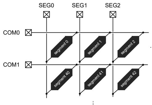
**Note:** In order to avoid degradation due to electrophoresis in the liquid crystal, the waveform of the voltage across a segment must not have a DC component.
