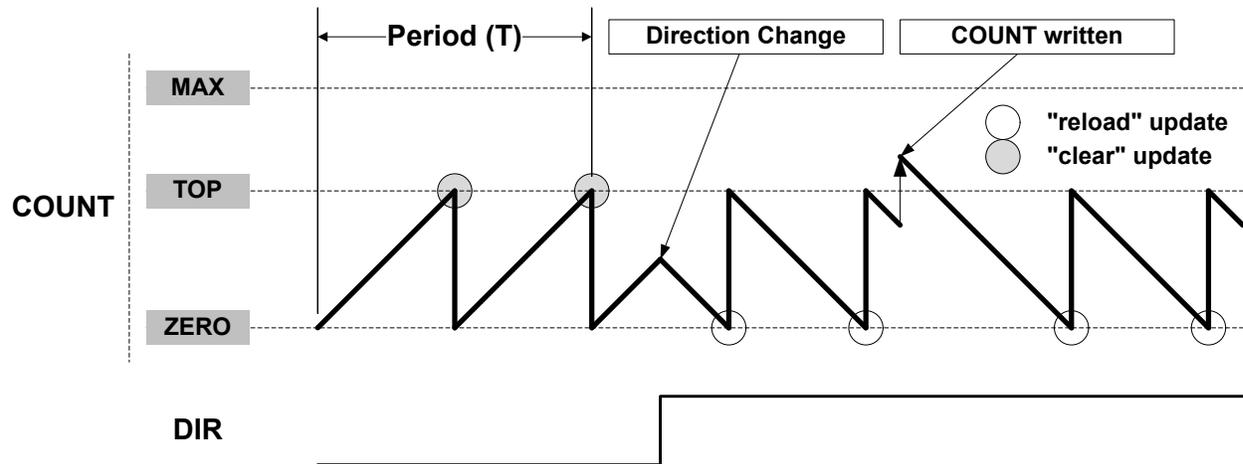
Due to asynchronous clock domains, the internal counter settings are written when the synchronization is complete. Normal operation must be used when using the counter as timer base for the capture channels.
