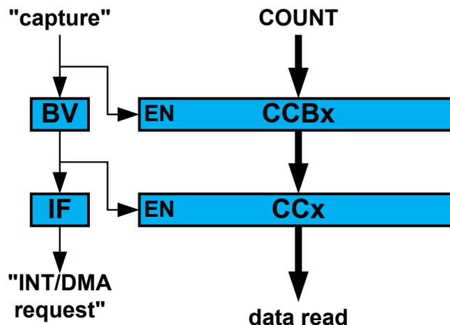
For input capture, the buffer register and the corresponding CCx act like a FIFO. When CCx is empty or read, any content in CCBUFx is transferred to CCx. The buffer valid flag is passed to set the CCx interrupt flag (IF) and generate the optional interrupt, event or DMA request. CCBUFx register value can't be read, all captured data must be read from CCx register.
