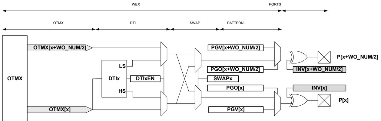
The output matrix (OTMX) unit distributes compare channels, according to the selectable configurations in Table 35-4.
