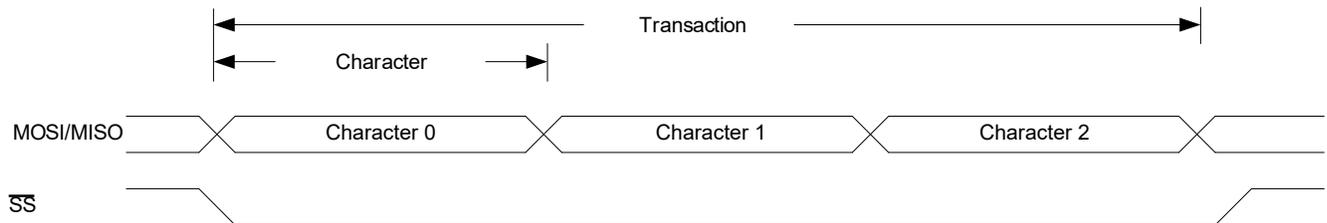
The SPI Host must pull the SPI Select line ( $\overline{SS}$ ) of the desired Client low to initiate a transaction. The Host and Client prepare data to send via their respective shift registers, and the Host generates the serial clock on the SCK line.
