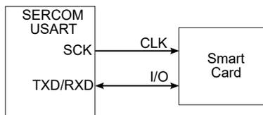
ISO 7816 characters are specified as 8 bits with even parity. The USART must be configured accordingly.
