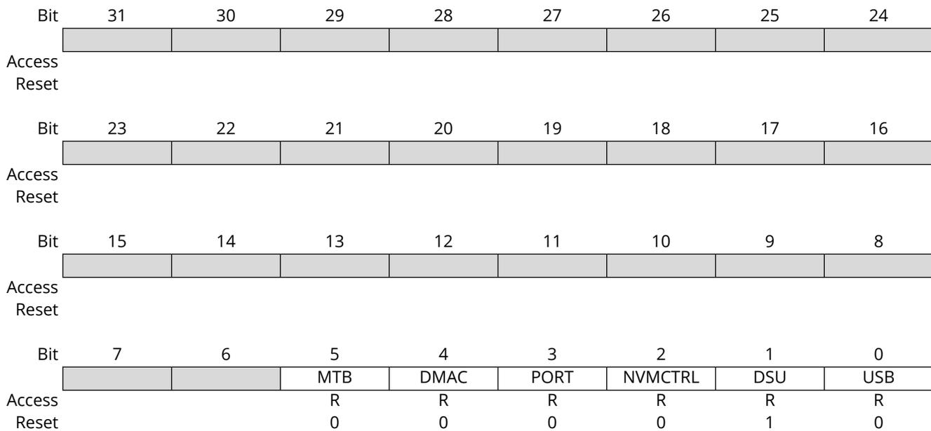
**Bit 5 - MTB** Peripheral MTB Write Protection Status
