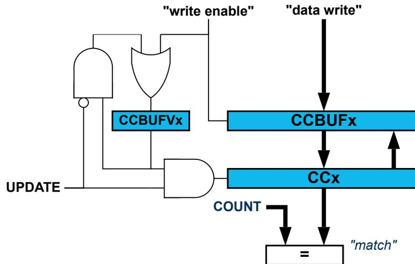
Both the registers (PER/CCx) and corresponding buffer registers (PERBUF/CCBUFx) are available in the I/O register map, and the double buffering feature is not mandatory. The double buffering is disabled by writing a '1' to CTRLBSET.LUPD.
