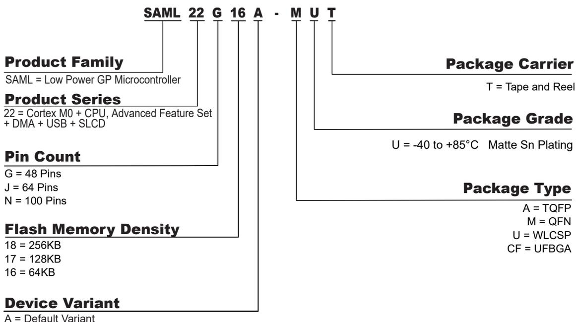
**Note:** The device variant (last letter of the ordering number) is independent of the die revision (DSU.DID.REVISION); The device variant denotes functional differences, whereas the die revision marks evolution of the die.
