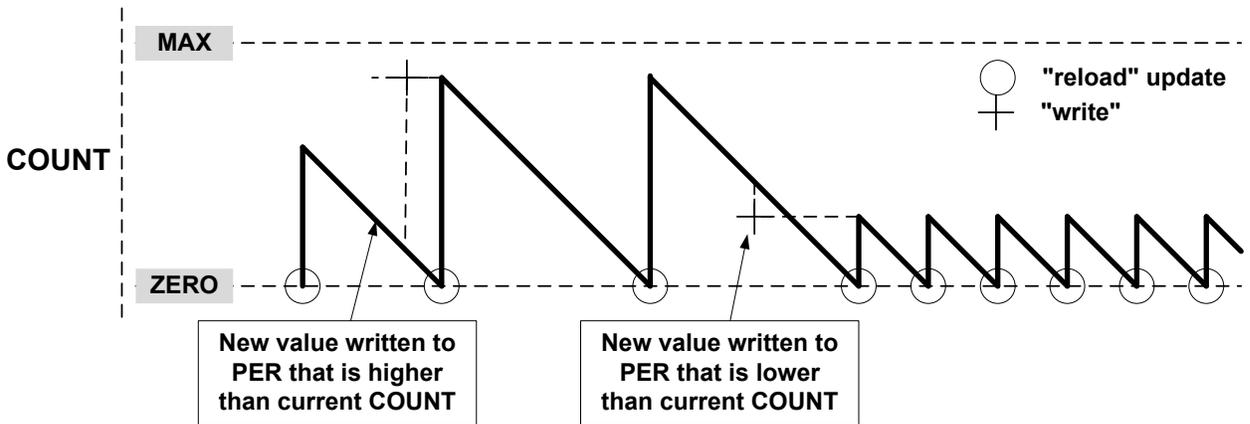
A counter wraparound can occur in any operation mode when up-counting without buffering, see the following figure. COUNT and TOP are continuously compared, so when a new value that is lower than the current COUNT is written to TOP, COUNT will wrap before a compare match.
