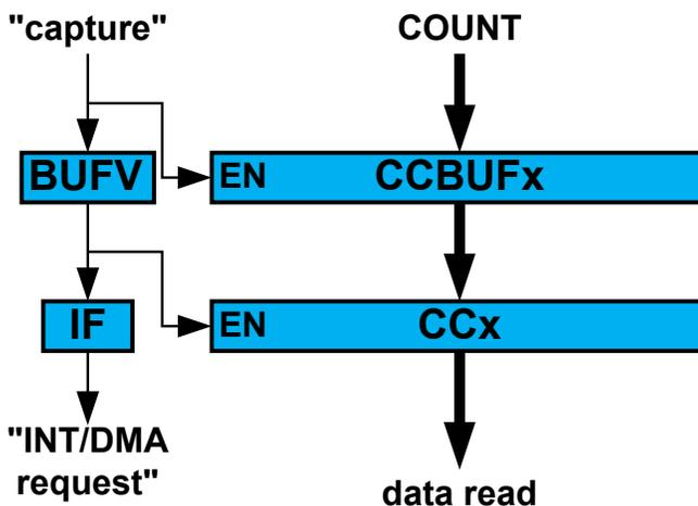
The TCC can detect capture overflow of the input capture channels: When a new capture event is detected while the Capture Buffer Valid flag (STATUS.CCBUFVx) is still set, the new timestamp will not be stored and INTFLAG.ERR will be set.
