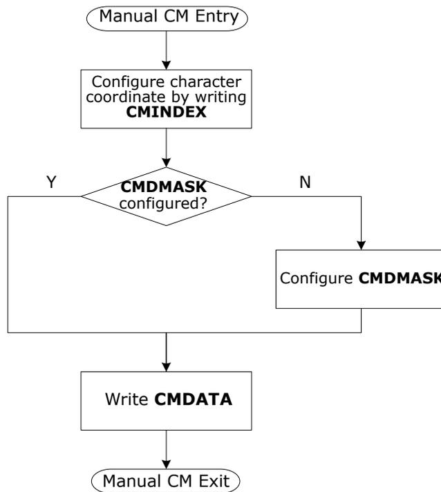
By this character mapping feature, user could update any particular rectangular window defined by CMCFG and CMINDEX in the display memory just by a single APB write access.
