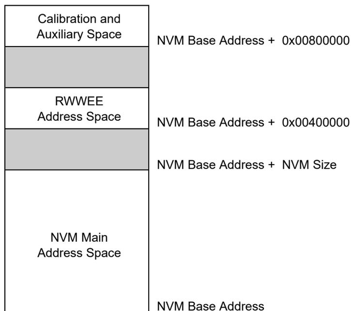
The lower rows in the NVM main address space can be allocated as a boot loader section by using the NVM User Row BOOTPROT fuses, and the upper rows can be allocated to EEPROM Emulation section by using the NVM User Row EEPROM fuses, as shown in the following figure.
