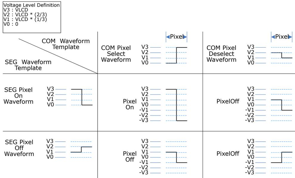
Figure 42-11. 1/3 Bias, 1/4 Duty, Standard Waveform
