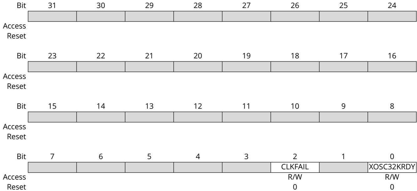
**Bit 2 – CLKFAIL** XOSC32K Clock Failure Detection
