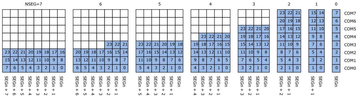
The 24 segments value is updated by a write access to the Character Mapping Segments Data register (CMDATA).
