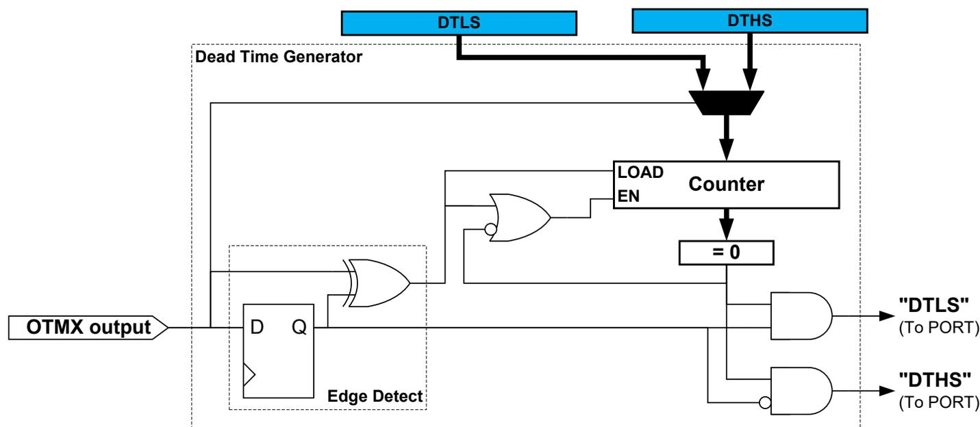
As shown in [Figure 35-36](#), the 8-bit dead-time counter is decremented by one for each peripheral clock cycle until it reaches zero. A non-zero counter value will force both the low side and high side
