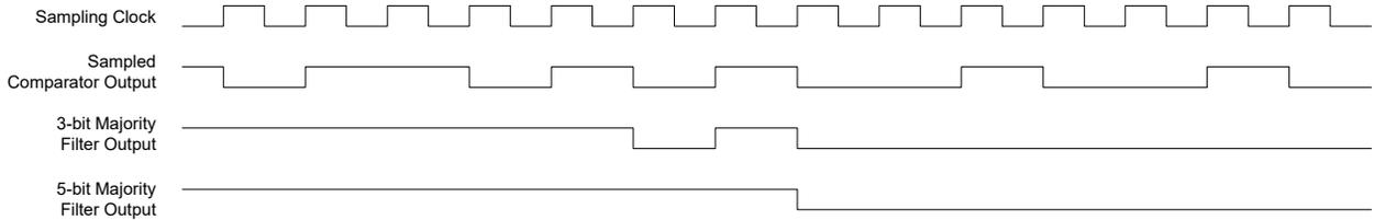
**Figure 41-7. Single-Shot Filtering**
