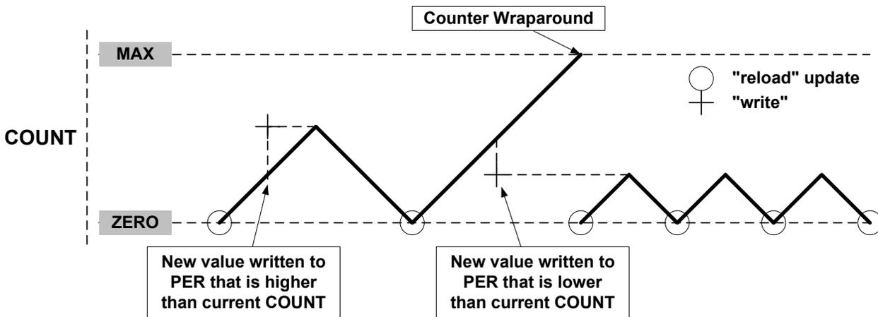
When double buffering is used, the buffer can be written at any time and the counter will still maintain correct operation. The period register is always updated on the update condition, as shown in the following figure. This prevents wraparound and the generation of odd waveforms.
