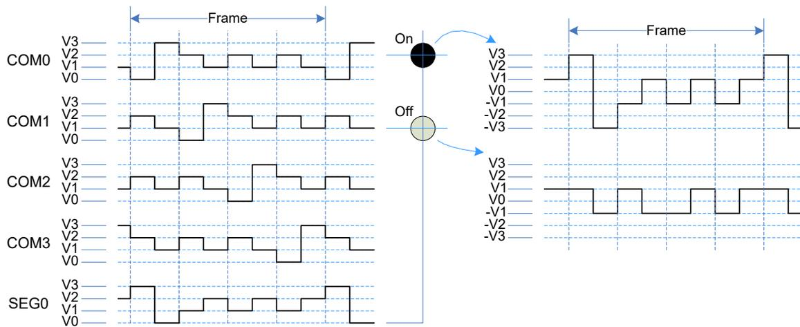
Figure 42-12. 1/3 Bias, 1/4 Duty, Low-Power Waveform
