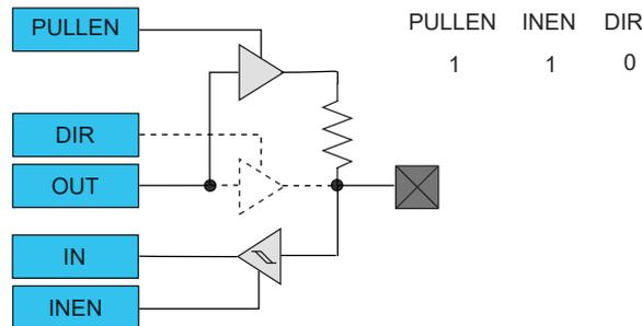
**Note:** When pull is enabled, the pull value is defined by the OUT value.
