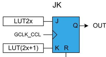
When the even LUT is disabled (LUTCTRL0.ENABLE=0 / LUTCTRL2.ENABLE=0), the flip-flop is asynchronously cleared. The reset command (R) is kept enabled for one APB clock cycle. In all other cases, the flip-flop output (OUT) is refreshed on rising edge of the GCLK\_CCL, as shown in the following table.
