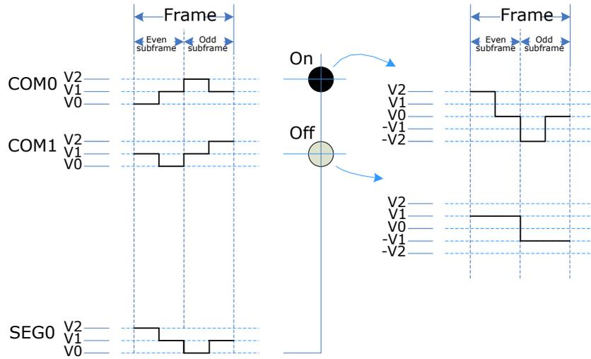
Figure 42-10. 1/3 Bias Standard Driving Waveform Template and Combination
