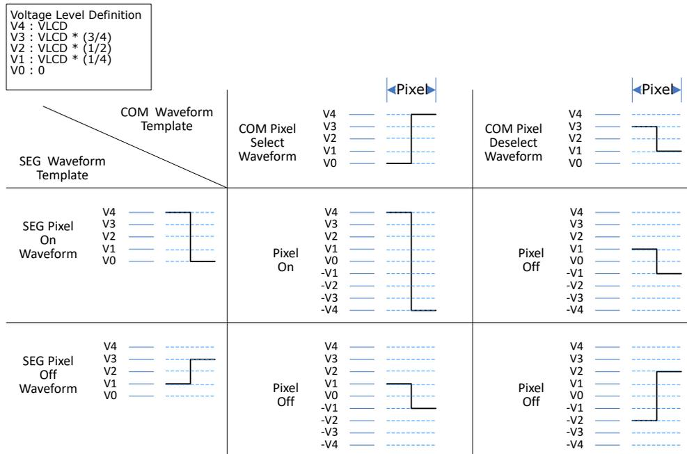
Figure 42-14. 1/4 Bias, 1/8 Duty, Standard Waveform
