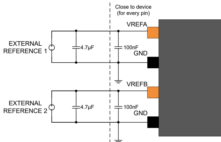
**Figure 47-5.** External Analog Reference Schematic With One Reference
