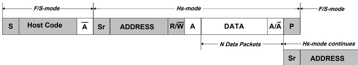
Transmitting in High-speed mode requires the I<sup>2</sup>C Host to be configured in High-speed mode (CTRLA.SPEED=0x2) and the SCL clock stretch mode (CTRLA.SCLSM) bit set to '1'.
