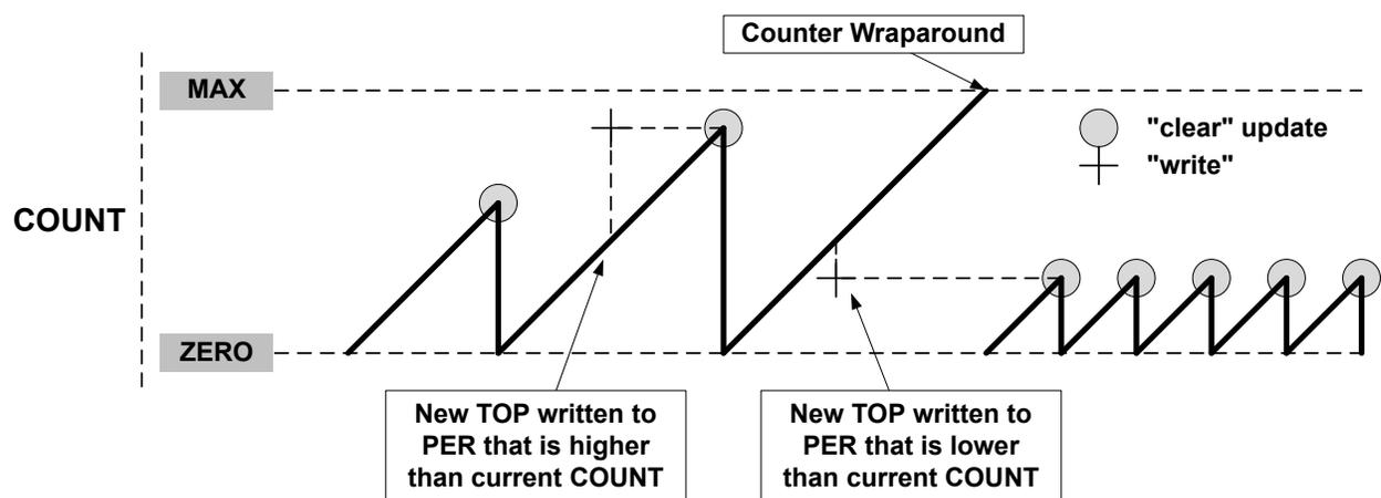
A counter wraparound can occur in any operation mode when up-counting without buffering, see [Figure 34-8](#).
