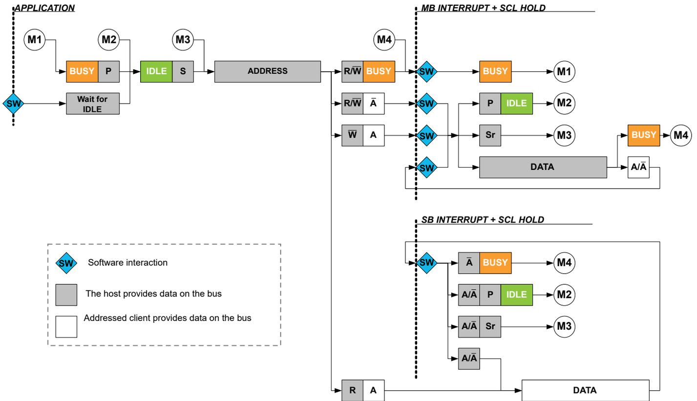
In the second strategy (CTRLA.SCLSM=1), interrupts only occur after the ACK bit, as in [Host Behavioral Diagram \(SCLSM=1\)](#). This strategy can be used when it is not necessary to check DATA before acknowledging.
