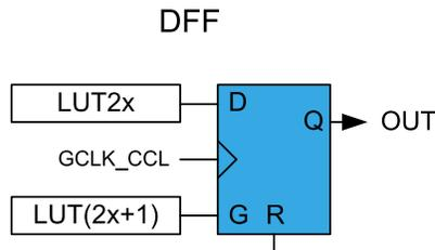
When the even LUT is disabled (LUTCTRL0.ENABLE=0 / LUTCTRL2.ENABLE=0), the flip-flop is asynchronously cleared. The reset command (R) is kept enabled for one APB clock cycle. In all other cases, the flip-flop output (OUT) is refreshed on rising edge of the GCLK\_CCL, as shown in the following table.
