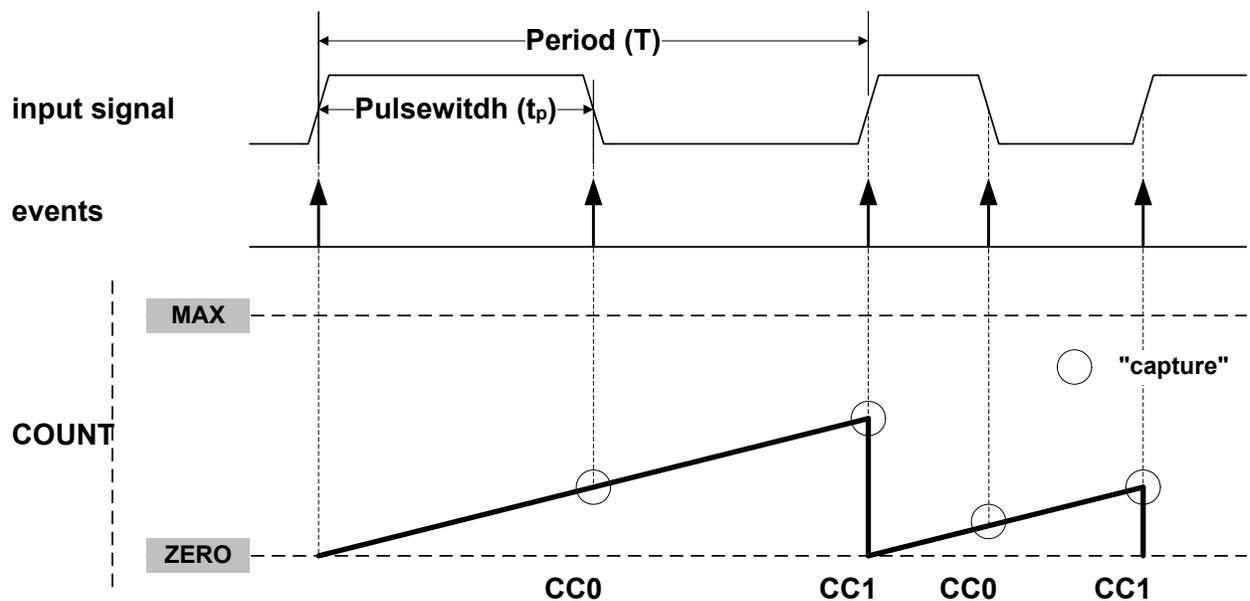
Selecting PWP in the Event Action bit group in the Event Control register (EVCTRL.EVACT) enables the TC to perform one capture action on the rising edge and the other one on the falling edge. The period  $T$  will be captured into CC1 and the pulse width  $t_p$  in CC0. EVCTRL.EVACT=PPW (period and pulse-width) offers identical functionality, but will capture  $T$  into CC0 and  $t_p$  into CC1.
