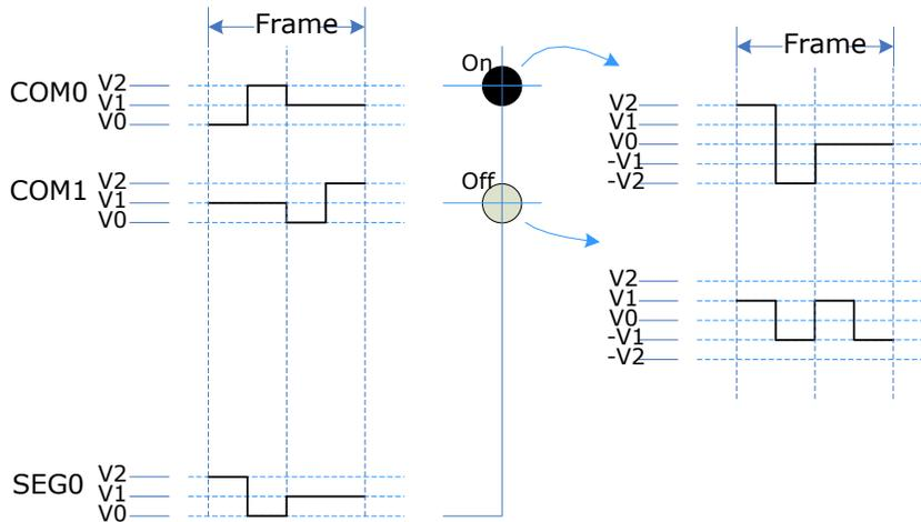
The low-power waveform template can be derived from the standard one by separating the standard waveform template into two subframe templates, as shown in the following figure:
