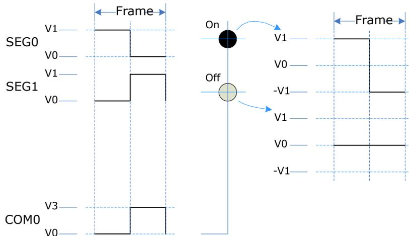
Figure 42-6. 1/2 Bias Waveform Template
