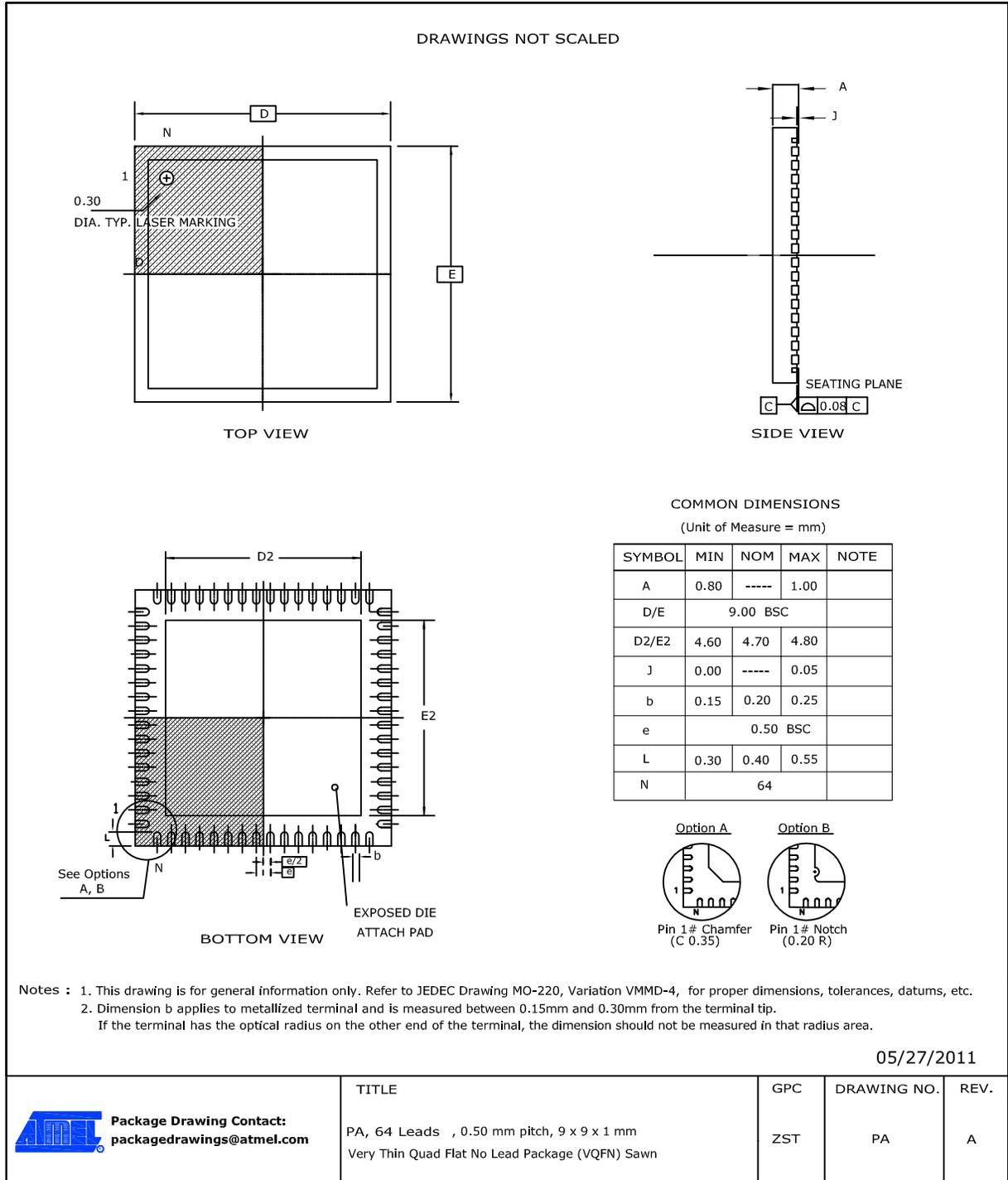
**Note:** It is recommended that the exposed pad be connected to ground in the PCB.
