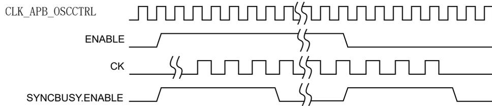
The frequency of the DPLL output clock CK is stable when the module is enabled and when the Lock bit in the DPLL Status register is set (DPLLSTATUS.LOCK).
