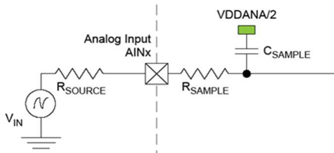
The minimum sampling time  $t_{SAMPLEHOLD}$  for a given  $R_{SOURCE}$  can be found using this formula:
