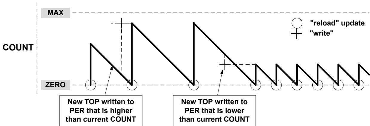
When double buffering is used, the buffer can be written at any time and the counter will still maintain correct operation. The period register is always updated on the update condition, as shown in Figure 34-10. This prevents wraparound and the generation of odd waveforms.
