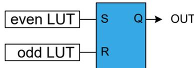
When the even LUT is disabled (LUTCTRL0.ENABLE=0 / LUTCTRL2.ENABLE=0), the latch output will be cleared. The R-input is forced enabled for one more APB clock cycle and S-input to zero. In all other cases, the latch output (OUT) is refreshed as shown in the following table.
