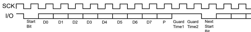
If a parity error is detected by the receiver, it drives the I/O line to 0 during the guard time, as shown in the next figure. This error bit is also named NACK, for Non Acknowledge. In this case, the character lasts 1 bit time more, as the guard time length is the same and is added to the error bit time, which lasts 1 bit time.
