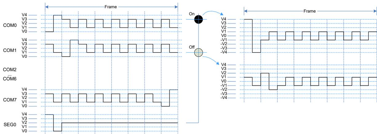
Figure 42-15. 1/4 Bias, 1/8 Duty, Low-Power Waveform
