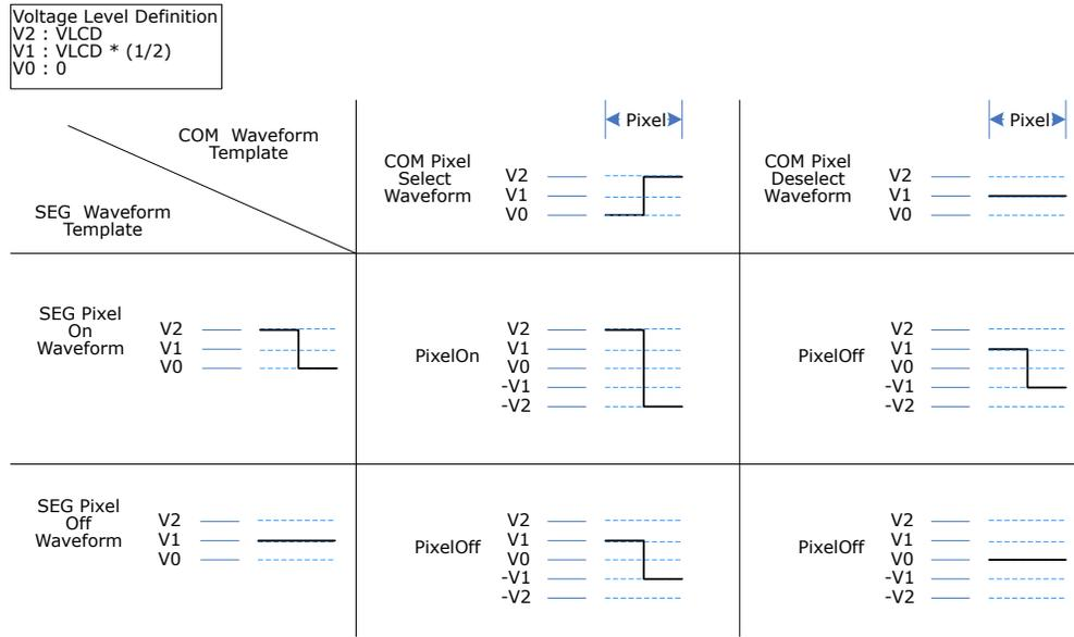
Figure 42-7. 1/2 bias, 1/2 Duty Standard Waveform
