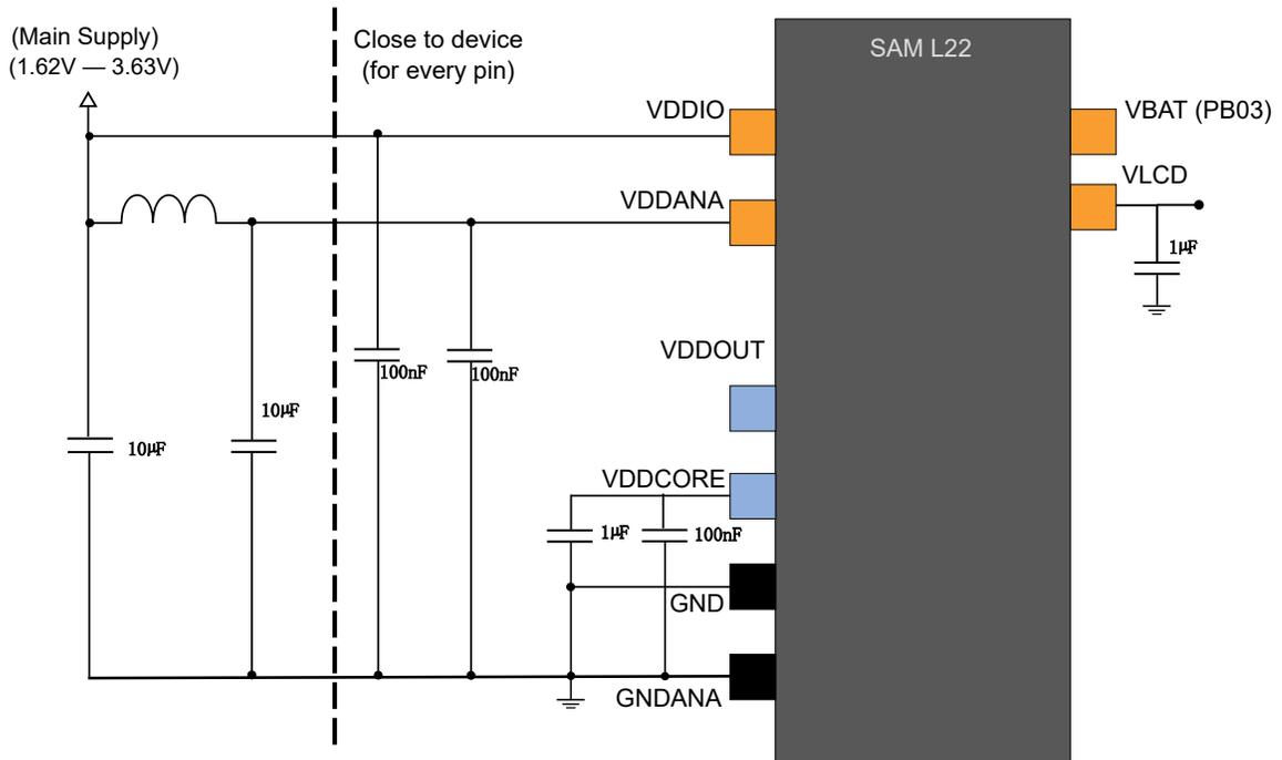
Figure 47-3. Power Supply Connection for Battery Backup
