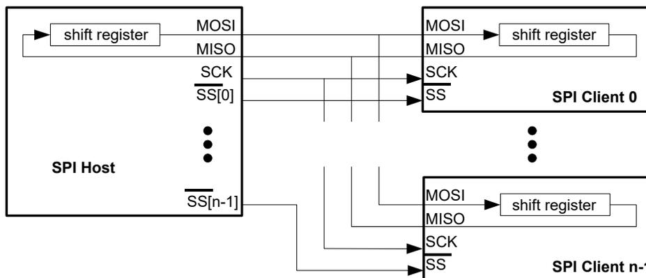
Another configuration is multiple Clients in series, as in [Multiple Clients in Series](#). In this configuration, all n attached Clients are connected in series. A common  $\overline{SS}$  line is provided to all Clients, enabling them simultaneously. The Host must shift n characters for a complete transaction. Depending on the Host SPI Select Enable bit (CTRLB.MSSEN), the  $\overline{SS}$  line can be controlled either by hardware or user software and normal GPIO.
