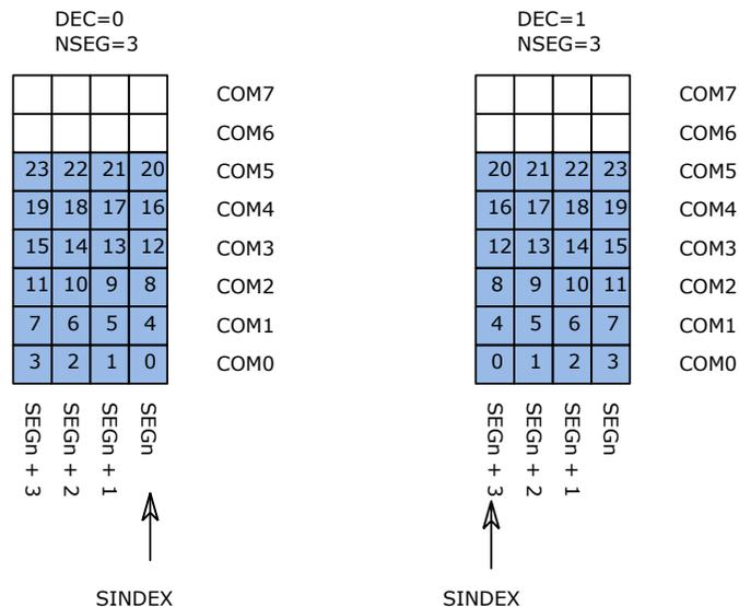
**Note:** The user must make sure all character bits could be mapped to some bit in display memory, not somewhere out side display memory.
