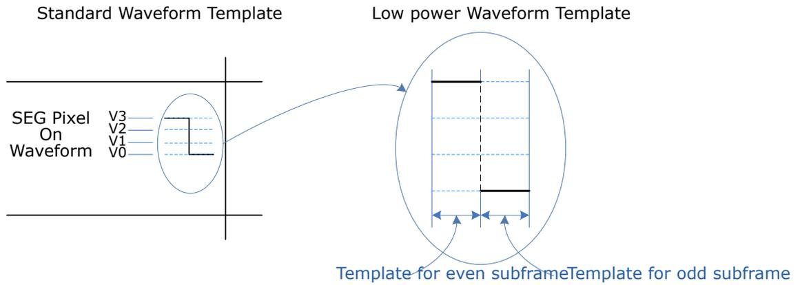
**Figure 42-9.** 1/2 Bias, 1/2 Duty Low-Power Waveform
