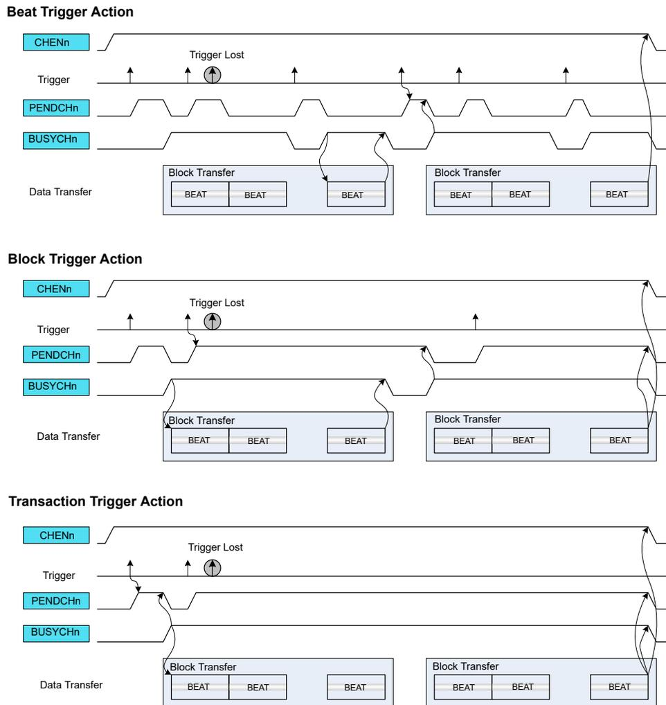
If the trigger source generates a transfer request for a channel during an ongoing transfer, the new transfer request will be kept pending (CHSTATUS.PEND=1), and the new transfer can start after the ongoing one is done. Only one pending transfer can be kept per channel. If the trigger source
