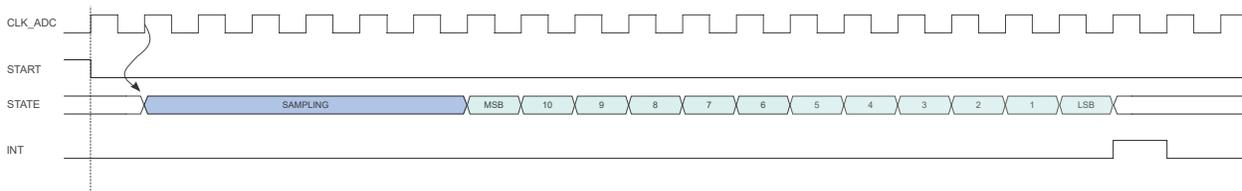
The ADC can also provide offset compensation, as shown in the following figure. The offset compensation is enabled by the Offset Compensation bit in the Sampling Control register (SAMPCTRL.OFFCOMP).
