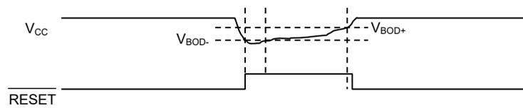
Enabling the BOD33 hysteresis by writing the Hysteresis bit in the BOD33 register (BOD33.HYST) to '1' will add hysteresis to the BOD33 threshold level.
