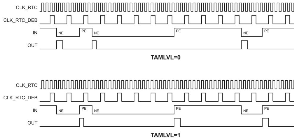
Figure 24-7. Edge Detection with Synchronous Stability Debouncing
