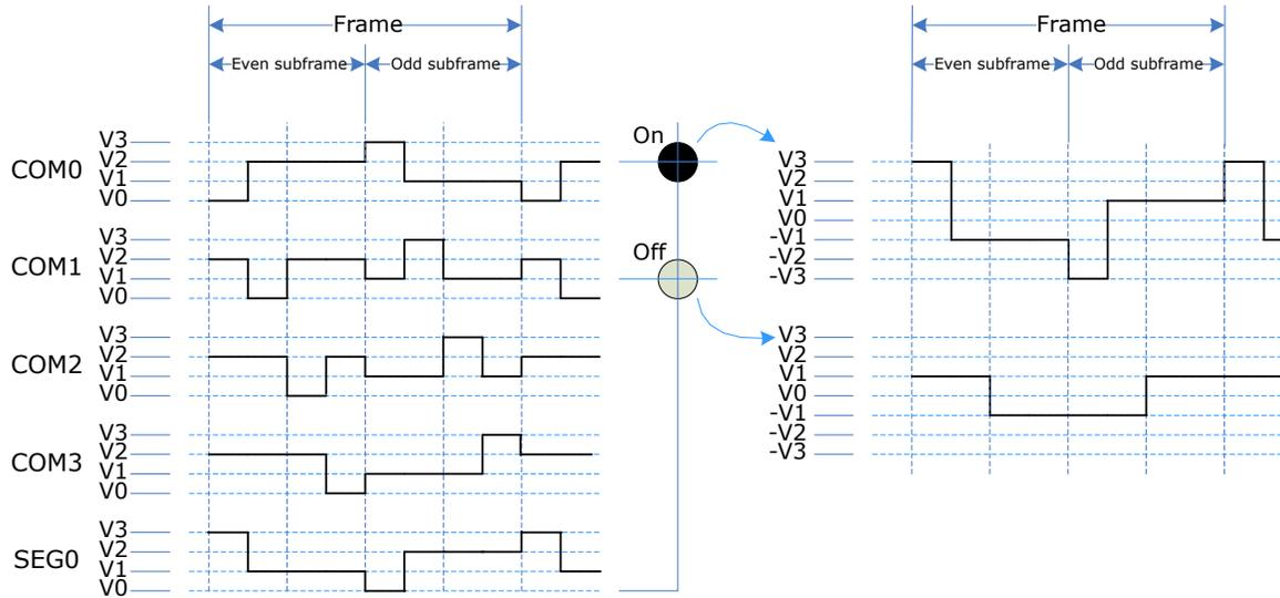
Figure 42-13. 1/4 Bias Standard Driving Waveform Template and Combination
