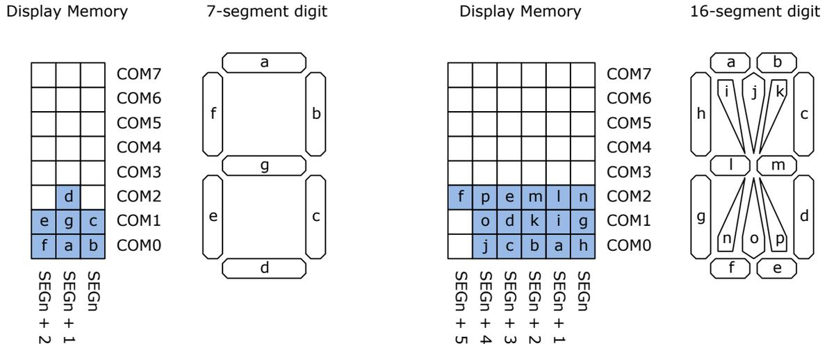
Several digits can be mapped in display memory to form a digits chain, which is used to display a characters string. Once configured, the user updates a digit by providing up to 24 bits with a single write access. ASCII tables provide standard symbols which should be handled by software before being displayed.
