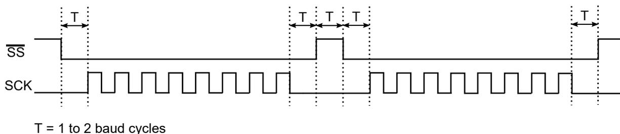
When CTRLB.MSEN=0, the  $\overline{SS}$  pin(s) is/are controlled by user software and normal GPIO.
