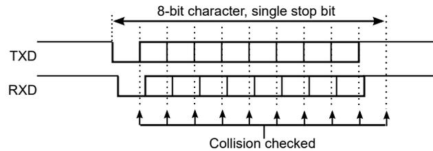
The next figure shows the conditions for a collision detection. In this case, the start bit and the first data bit are received with the same value as transmitted. The second received data bit is found to be different than the transmitted bit at the detection point, which indicates a collision.
