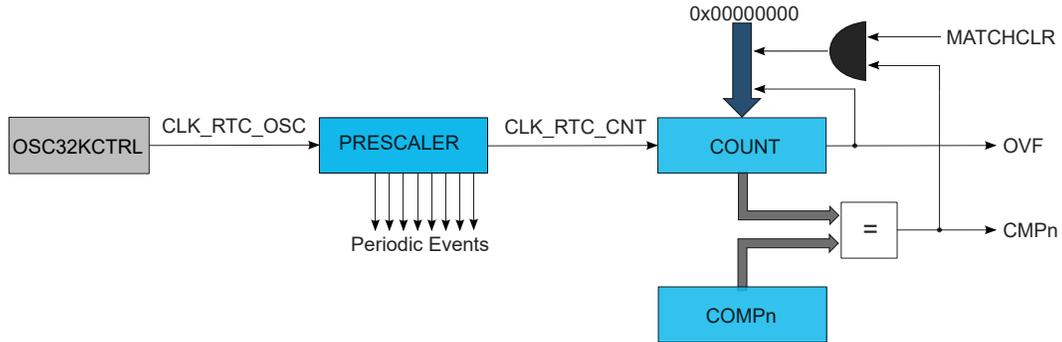
Figure 24-2. RTC Block Diagram (Mode 1 — 16-Bit Counter)
