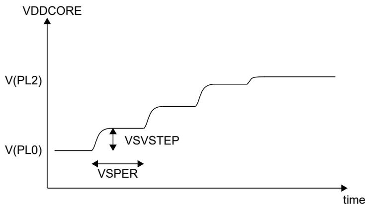
Setting VREG.VSVSTEP to the maximum value allows to transition in one voltage step.
