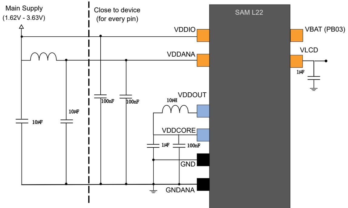
Figure 47-2. Power Supply Connection for Linear Mode Only
