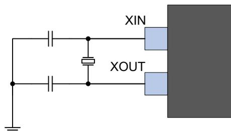
The crystal must be located as close to the device as possible. Long-signal lines may cause too high of a load to operate the crystal, and cause crosstalk to other parts of the system.
