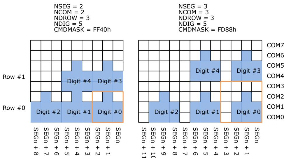
After the user has enabled ACM by writing a '1' to the ACM Enable bit in the Control C register (CTRLC.ACMEN), the ACM logic (state machine) will start according to the configuration by user. Whenever the user writes a '0' to CTRLC.ACMEN, the ACM logic will return to its initial state.
