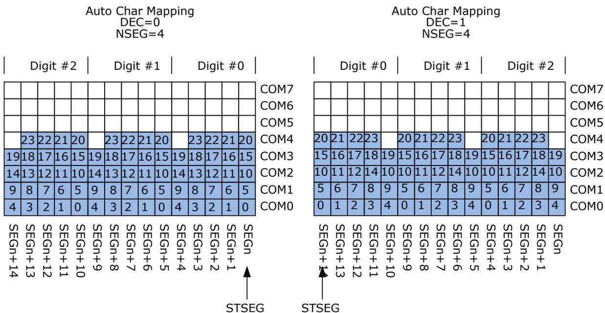
There are two usage models available under ACM, defined by the Mode bit in the Automated Character Mapping Configuration register (ACMCFG.MODE): when MODE=0, the *Sequential Characters String Display* mode is selected. When MODE=1, the *Scrolling of Characters String Display* mode is selected.
