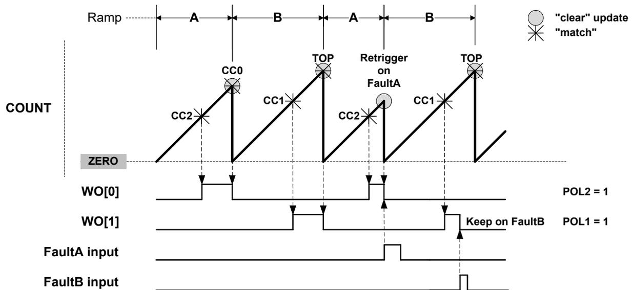
Figure 35-21. RAMP2 Critical Operation With 2 Channels
