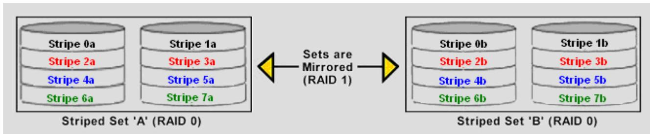
The data is written to RAID Group A, which is striped (RAID 0). This allows maximum speed. The data is then mirrored to another RAID 0 striped set, which is Set B in the figure above. This provides data redundancy (RAID 1), and thus increased data security.
