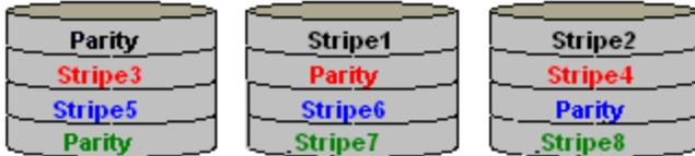
Parity RAID uses less capacity for protection and is the preferred method to reduce the cost per megabyte for larger installations. Mirroring requires 100% increase in capacity to protect the data whereas the above example only requires a 50% increase. The required capacity decreases as the number of disks in the group increases.
