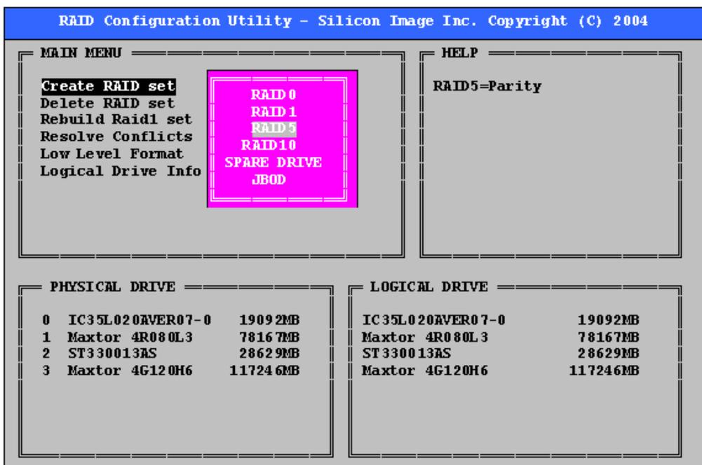
The Create RAID set option is also used to allocate a spare drive or a virtual drive (JBOD). The spare drive can be allocated to the set in the event of a failure of one of the drives in the set. To allocate a spare drive or JBOD, follow the procedure outlined above, choosing "SPARE DRIVE" or "JBOD" for the set type.
