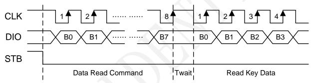
**A Note:** In the read mode, the PC next After the first eight of the rising edge of CLK key command when you want to read keys. The first falling edge of CLK data begins to be delayed a Twait latency (Twait =  $5\mu$ s)
