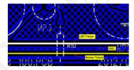
▲ Note: If LED control signals crossover sensor traces, it is recommended to use another plane jumper to cross lines instead of using SMT components. By doing this, the vertical distance between LED control signals and sensor traces will maintain in PCB thickness (1.6mm) to guarantee EFT immunity.
