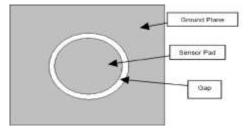
A typical round shape sensor pad is illustrated above. There is a round gap that isolates the sensor pad and the ground plane.
