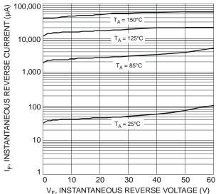
Figure 3 Typical Reverse Characteristics
