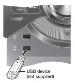
1 Lower the volume and connect the USB device to the USB port.
