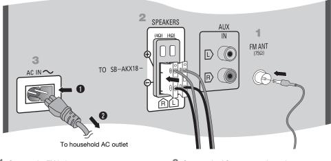
**1** Connect the FM indoor antenna. Put the antenna where there is the best reception.
