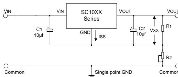
$$V_{OUT} = V_{xx} \cdot \left( 1 + \frac{R_2}{R_1} \right) + I_{ss} \cdot R_2$$
