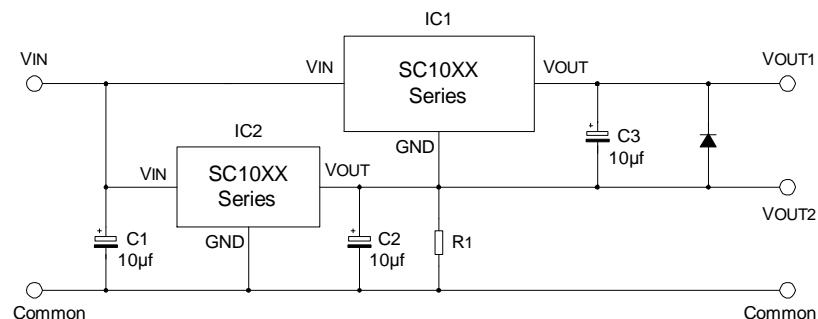
Note: The circuit and parameters are reference only, please set the parameters of the real application circuit based on the real test .
