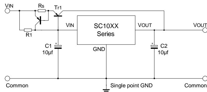
Circuit for increasing output voltage
