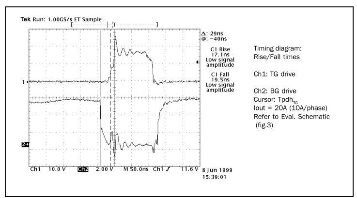
$V_{IN} = 12V, V_{OUT} = 1.6V.$  Top FET = IR7811 FDB7030(BL) Qgd = 23nc
