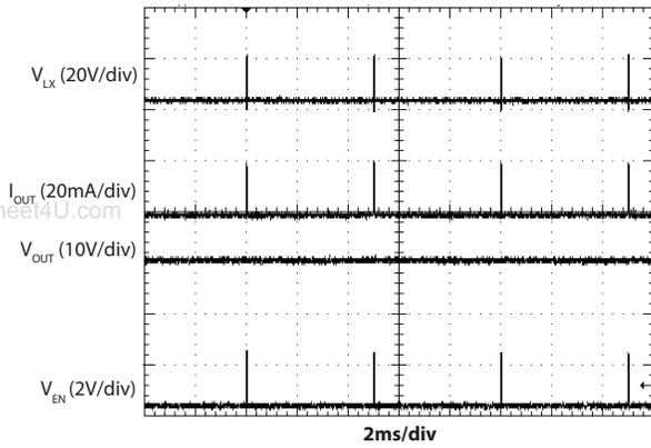
PWM Operation at 50kHz and 15% Duty Cycle
