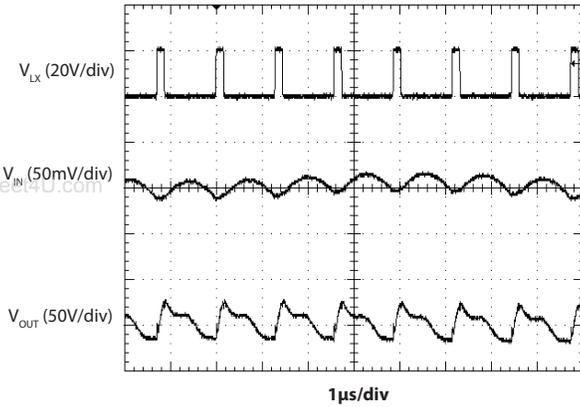
Typical Waveforms at  $V_{IN} = 5.5V$
