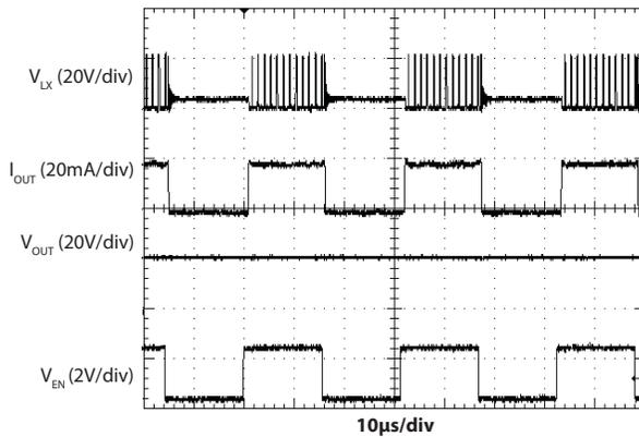
PWM Operation at 32kHz and 10% Duty Cycle
