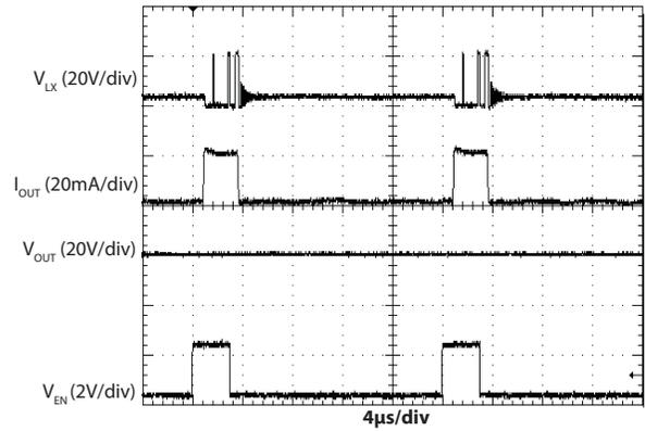
PWM Operation at 32kHz and 50% Duty Cycle
