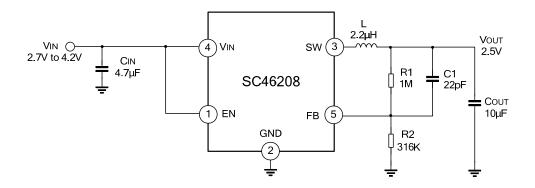
Fig. 1: Output voltage adjustable regulator, single battery to 2.5V converter
