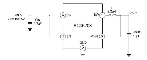
Fig.2: Output voltage fixed regulator
