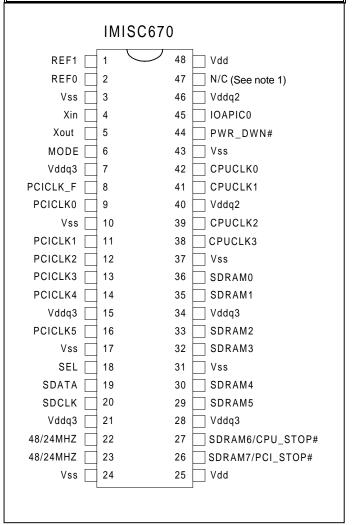
Note 1: N/C is a no connect pin. IMI product does <u>not</u> require CPU 3.3\_2.5# select line to operate properly at 2.5 volts. This pin may be connected externally to Vdd or Vss.
