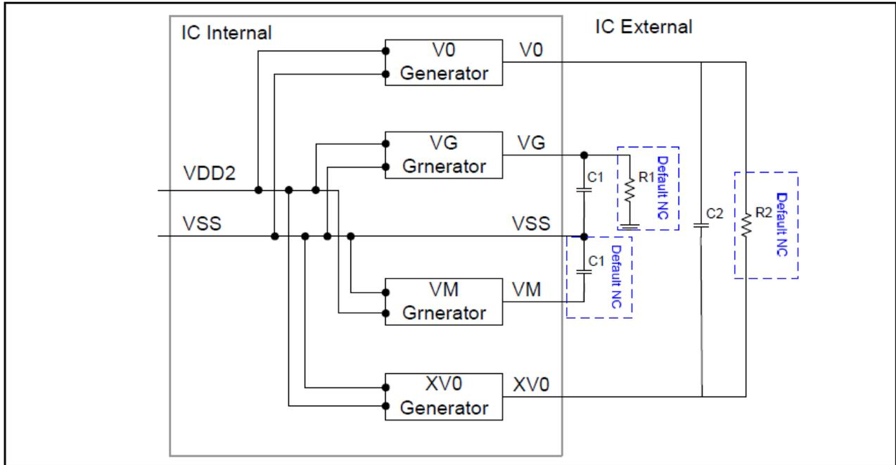
**Fig 10 Power Circuit**
