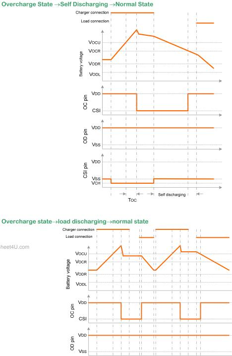
$Overcharge \ state {\rightarrow} load \ discharging {\rightarrow} normal \ state$ Charger connection Load connection www.DataSheet4U.com Battery voltage
