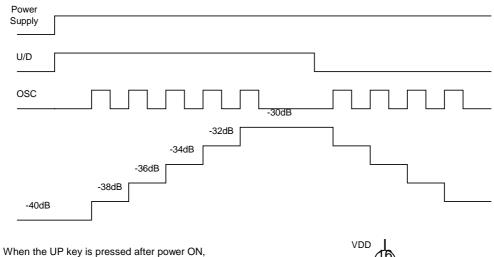
When the UP key is pressed after power ON the U/D terminal is place in the UP state at "H" level, and the oscillator is actuated. When the DOWN key is pressed, the U/D terminal is kept at "L" level as long as the Down key is pressed, and the oscillator is actuated in the down state and therefore, attenuation is decreased. Oscillation frequency is decided by Cx and Rx.
