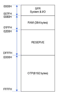
SFR: Special function registers. This block includes system control & status register and the mapping of ports and display data block.
