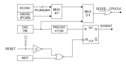
The system reset occurs when: internal watchdog counting overflows; external Reset pin input low level. The circuit jumps to the start address of the program from reset address FFFAH and begins working normally.
