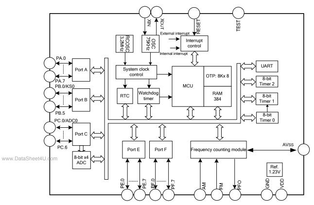
Note: Pin VPP can be diplexed as RESET, when program the OTP memory, this pin is connected to 12V.
