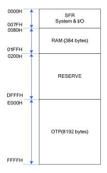
SFR: Special function registers. This block includes system control, state register and the mapping of ports and display data block.
