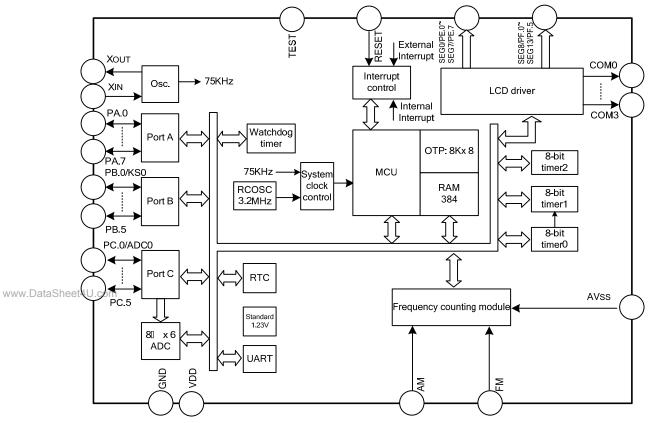
Note: VPP pin can be diplexed as RESET, when program the OTP memory, this pin is connected to 12V voltage.
