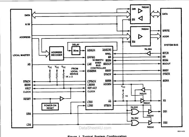
Figure 1. Typical System Configuration
