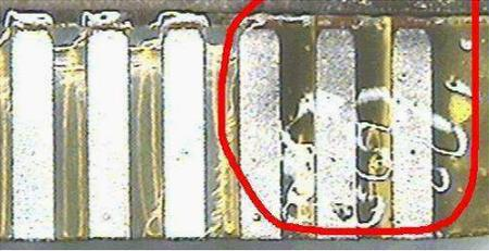
A photograph of several PCB pins. One pin is circled in red, showing a white, irregular substance (glue or contamination) on its surface.                                                                     |
