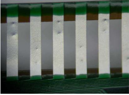
A photograph of a PCB terminal lead with a small, dark mark on its surface, which is identified as a prober mark.                                                                                             |
