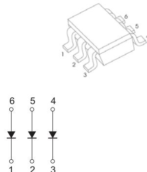
**MARKING: KLL****Maximum Ratings and Electrical Characteristics, Single Diode @Ta=25°C**
