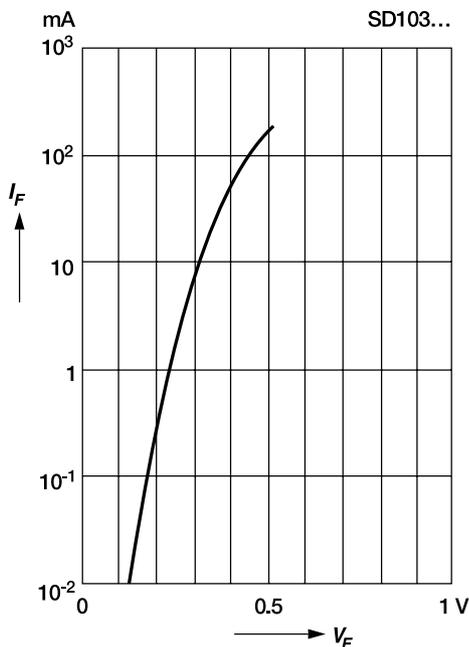
Typical high current forward conduction curve
