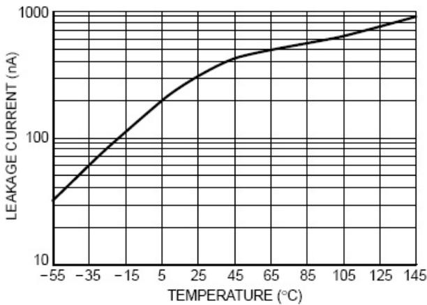
Figure 3. SD05 Typical Leakage Current versus Temperature
