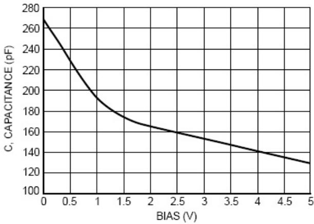
Figure 1. SD05 Typical Capacitance versus Bias Voltage
