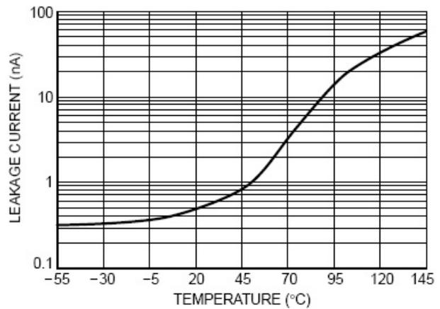
Figure 4. SD12 Typical Leakage Current versus Temperature
