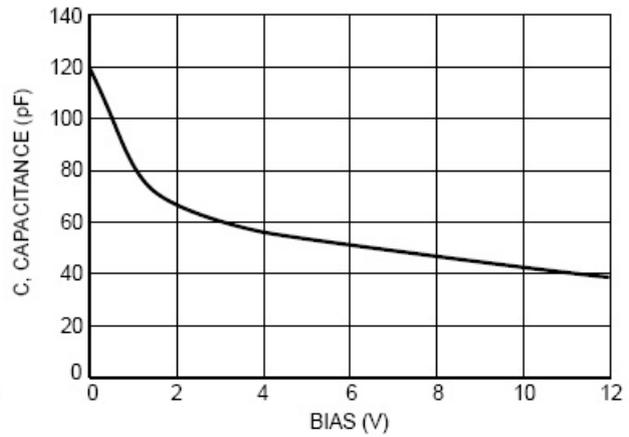
Figure 2. SD12 Typical Capacitance versus Bias Voltage
