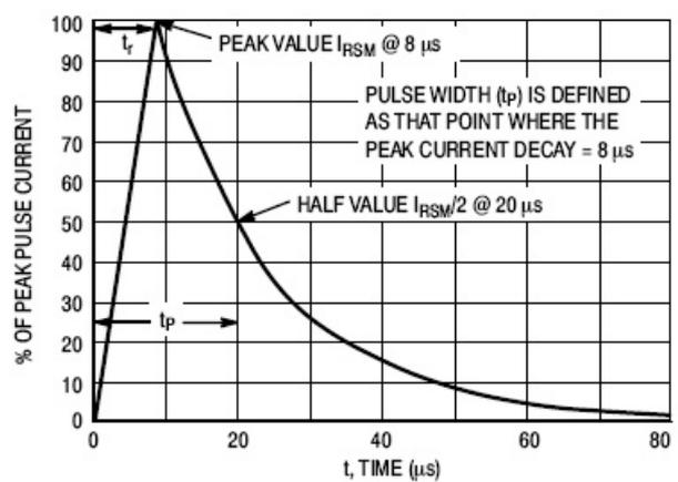
Figure 6. 8 x 20  $\mu s$  Pulse Waveform
