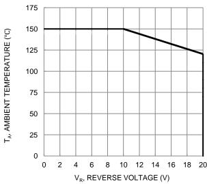
Figure 4. Operating Temperature Derating
