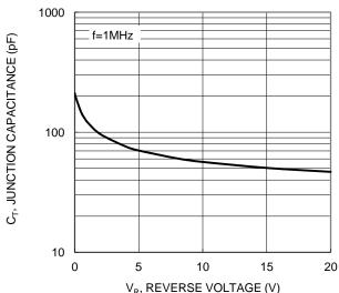
V<sub>R</sub>, REVERSE VOLTAGE (V) Figure 3. Typical Junction Capacitance
