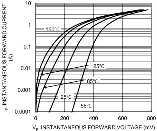
Figure 1. Typical Forward Characteristics
