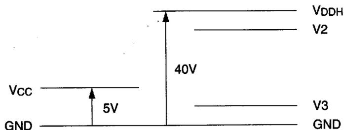
Note 2. If the logic circuit power supply comes to float power-supply voltage supply voltage is applied to the liquid crystal driving circuit, the LSI may be broken permanently. So, prevent the logic circuit power supply from floating.
