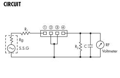
$Rg + R_1 = R_2 = Input/Output Impedance C = 10pF (Include stray capacitance)$
