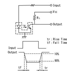
\*2 Method of Measuring Position Detection Characteristic
