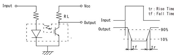
\*2 Method of Measuring Position Detection Characteristic
