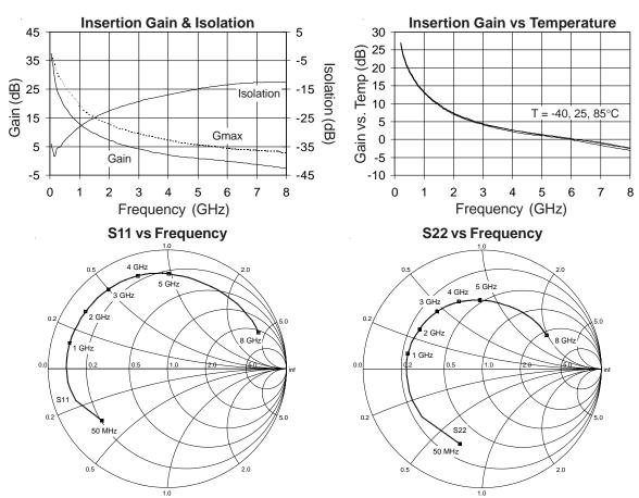
Note: S-parameters are de-embedded to the device leads with  $Z_s = Z_t = 50\Omega$ . The data represents typical performace of the device. De-embedded s-parameters can be downloaded from our website (www.sirenza.com).
