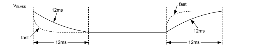
Figure 3. V ELVSS Transition Time Control
