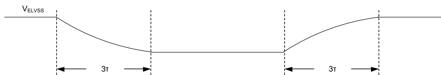
Figure 6. VELVSS Transition Time Control
