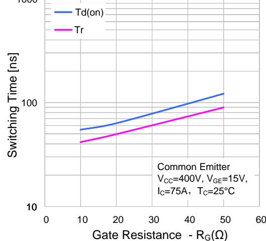
Figure 12. Turn-On Characteristic vs. Gate Resistance
