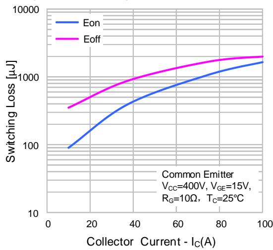
Figure 22. Switching Loss vs. Collector Current
