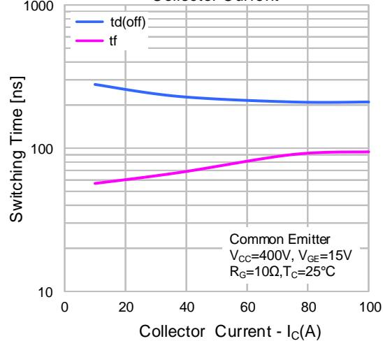
Figure 20. Turn-off Characteristic vs.
