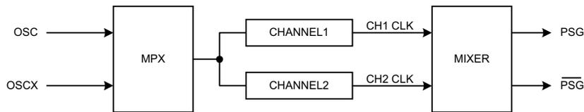
The PSG function provides four subfunctions for wide applications.
