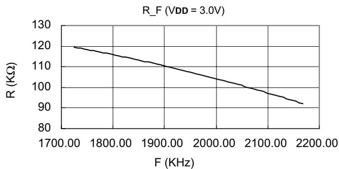
Figure 8. Resistor vs. F<sub>oscx</sub>
