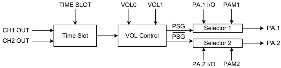
The MIXER mixes CH1-OUT and CH2-OUT into one single tone output to PA.1、PA.2, when PAM1 = 1、PAM2 = 1. Then the tone output is controlled by the volume control bit into 4 volume levels and in the end outputted by PSG.
