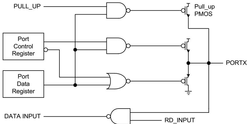
I/O ports of SH66P13A can be accessed by read/write system register. User can output any value to any I/O port bit at any time. Bit3 of the PMOD register controls On/Off of all pull-ups MOS simultaneously. Pull-up MOS is also controlled by the port data registers (PA, PB) of each port also. So the pull-up MOS can be turned On/Off.
