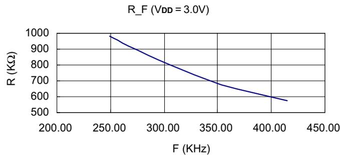
Figure 7. Resistor vs. F<sub>osc</sub>
